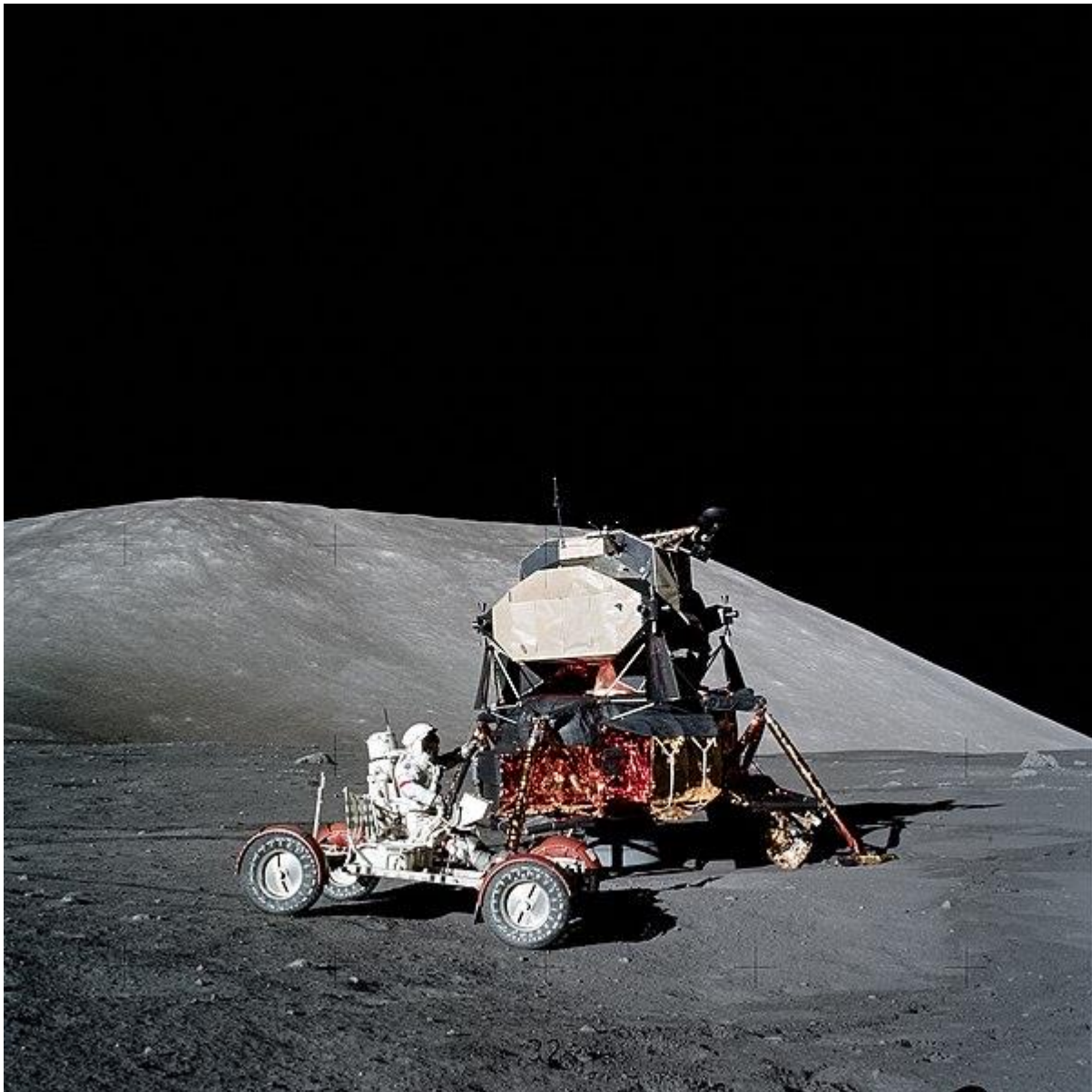
Figure 8. Eugene Cernan tests the lunar rover during the first Apollo 17 EVA on the surface of the Moon. The rover in foreground was deployed from the lander belly after touchdown. Such structures are classified as Type 1 habitats. [7]
