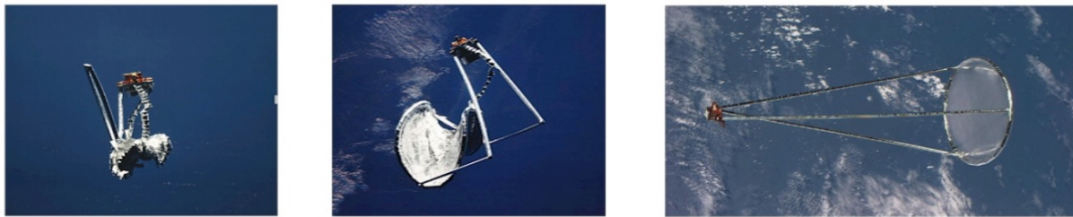
Figure 3. Antenna Inflating after deployment from STS77
