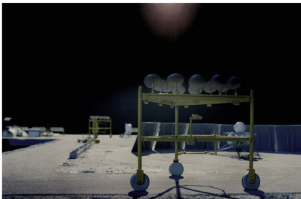
Fig. 5. Solar-powered Straddler mobile gantry offloads all Lander cargo, including itself.
