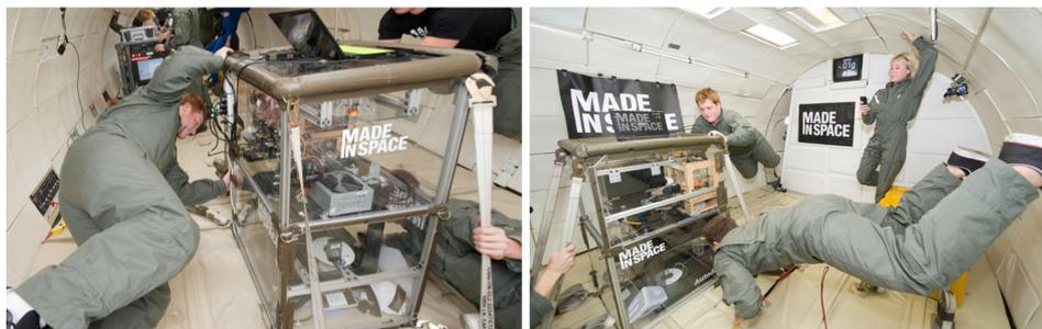
Fig. 5. 3D printing test in zero- and microgravity during a flight aboard a modified Boeing 727 from the Zero G Corporation. Left: A 'Made In Space' experiment box; right: A Microgravity Science Glovebox Engineering Unit. Courtesy of NASA (NASA, 2016).
