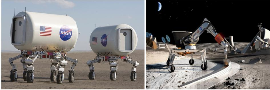
Fig. 2. ATHLETE and Contour Crafting: left: Two ATHLETE rovers used for field tests near Moses Lake, WA. (Boston.com, 2008), Image courtesy of NASA; right: Construction concept using the CC embedded on the ATHLETE (Khoshnevis and Zhang, 2012).
