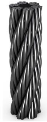
Figure 50: Stainless Steel Wire Rope Cable 6x7-FC side view. Image: Certex
