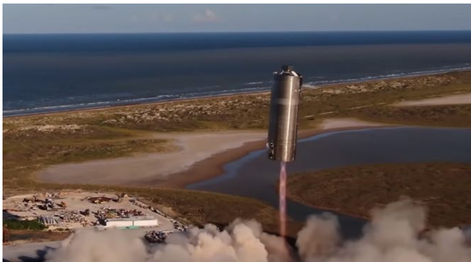
Figure 30: 150 meter hop of the Starship prototype SN-5. Photo: SpaceX
