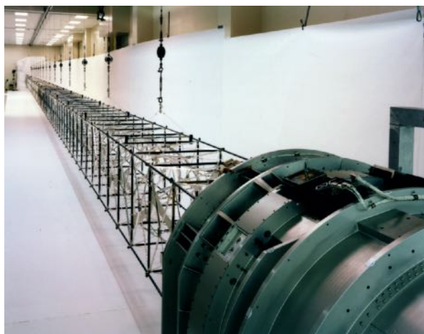
Figure 45: ADAM fully extended seen from the canister at AEC-Able Engineering. Image: AEC-Able Engineering
