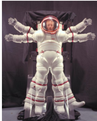
FIGURE 0. AX-5 “Hard” Spacesuit, mounted on the unpressurized donning fixture. The astronaut is evoking Da Vinci’s Vitruvian Man with his arms and legs. Designed by Hubert C. “Vic” Vykukal, Ames Research Center. NASA Photo.
