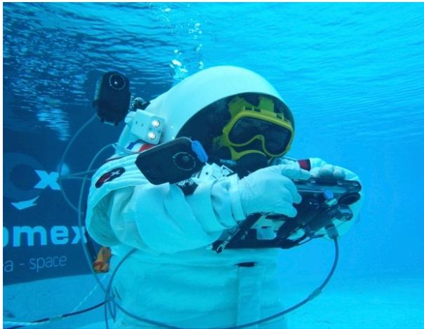
Fig. 11. The space suit simulator is operated underwater by a diver. It can be used to test various tools and control elements with the constraints of a pressurized suit. Photo credit: COMEX, 2016
