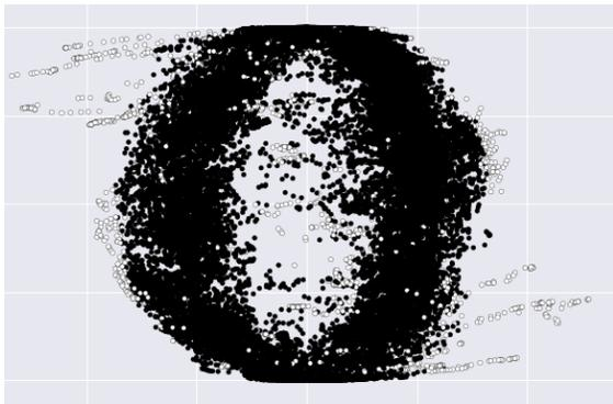
Fig. 13. Features extracted from accelerometer data. Filled black circles indicate ‘normal’ behaviour, unfilled circles indicate a hazardous condition.
