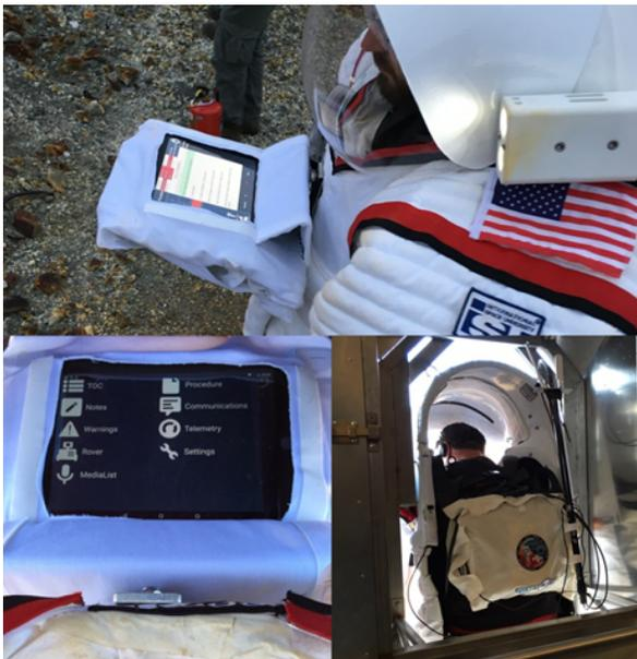
Fig. 12. EVA Information System (top, bottom left) and Suit Computer Assembly (bottom right), credit: Space Applications Services, 2016
