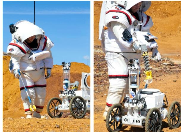
Fig. 14. Left: Sampling with the FPC, right: returning the sample in the rover Payload box with the PST, credit: Bruno Stubenrauch, 2016
