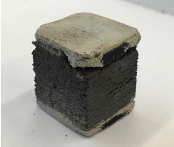
Figure 18 - Solar sintered sample, 20 \times 20 \times 20 mm 3 , used for compression tests, photo credit: DLR, 2017
