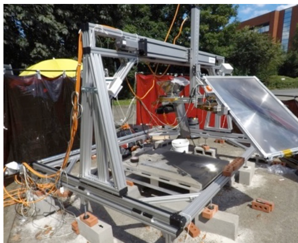
Figure 4 - Mobile 3D Printer System, credit: RegoLight Consortium, photo: LIQUIFER Systems Group, 2017
