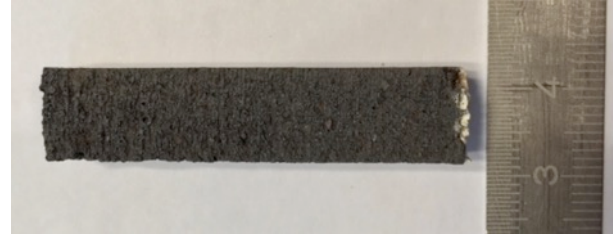
Figure 19 - Solar sintered sample used for bending test, photo credit: DLR, 2017
