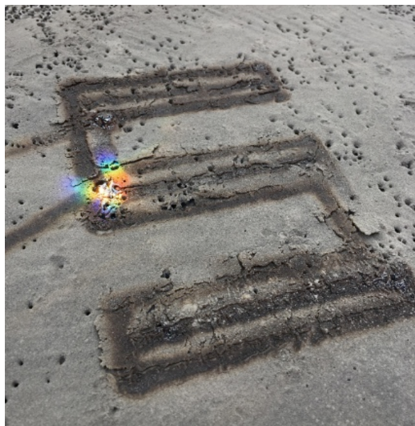
Figure 20 - Example of printed layer with enhanced resolution of mobile printing head, photo credit: Space Applications Services, 2017
