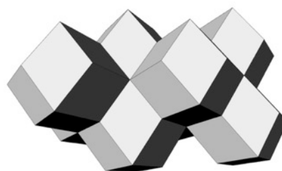
Figure 22 – Interlocking Element composed of rhombic dodecahedra developed for the August 2017 campaign.
