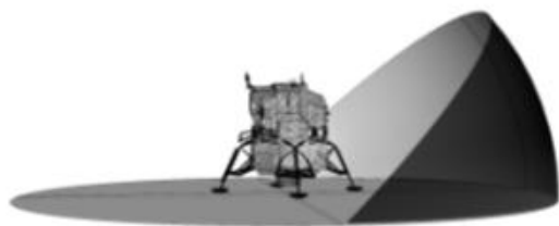
Figure 12: Launch pad with shield to protect against the dust created during the landing and launch sequence of a spacecraft. Credit: RegoLight consortium
