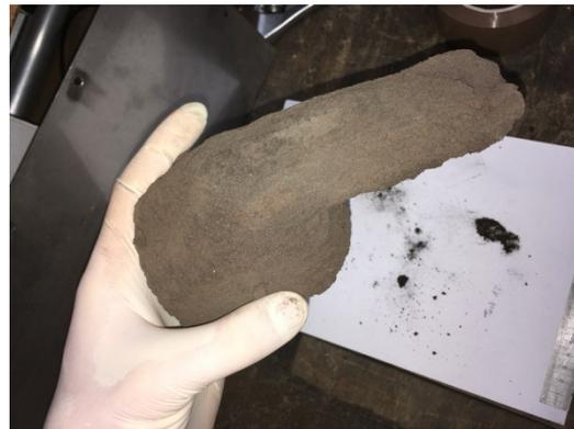
Figure 4: Computer designed interlocking building element (top) and actual sintered part (bottom), credit: RegoLight consortium, photo: DLR
