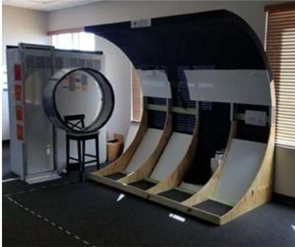
*Figure 2: Habitat Module Core Simulator 1/4 of 1:1*
