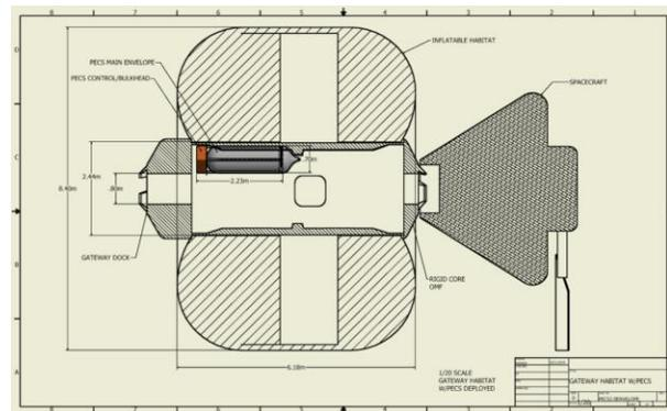
*Figure 4: 2D Habitat Module w/PECS Deployed*
