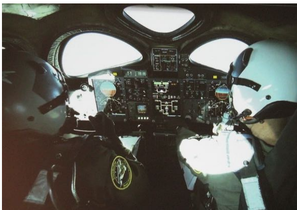
FIGURE 4b. SpaceShipTwo cockpit controls and displays and the forward windows. Courtesy of Virgin Galactic.
