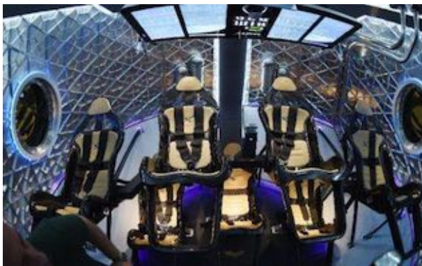
FIGURE 7b. SpaceX Crew Dragon V2 spacecraft interior view, showing seating for seven crew. Courtesy of SpaceX
