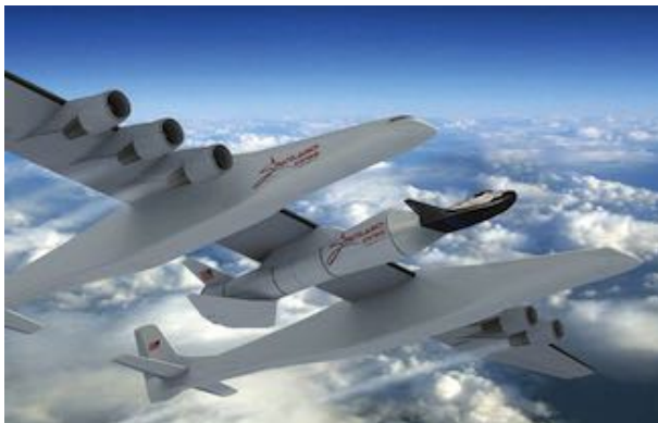
FIGURE 15a. Dream Chaser mounted on a "second stage" booster carried by the Stratolaunch aircraft. Courtesy of Sierra Nevada Corporation.
