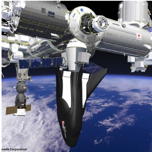
FIGURE 18. This CAD rendering from Sierra Nevada Corporation shows the Dream Chaser docked “tail-first” to the nadir (“-Z-bar”) docking port on the Unity Node on ISS. Note the Soyuz spacecraft to the left in similar nadir docking position on the Russian segment. Courtesy of Sierra Nevada Corp.
