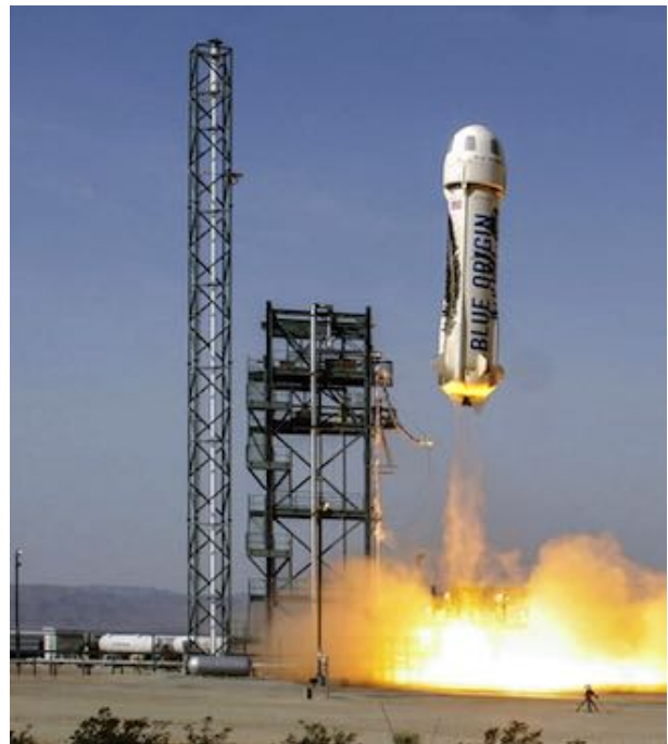
FIGURE 9. New Shepard launch, June 19, 2016 on a prototype single-stage suborbital rocket. This suborbital variant would perform a powered vertical landing. Courtesy of Blue Origin.
