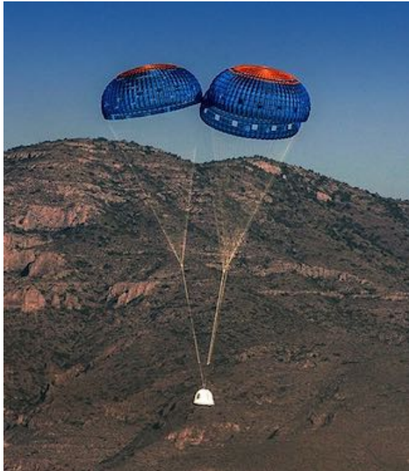
FIGURE 10. New Shepard capsule return parachute descent test. Courtesy of Blue Origin.
