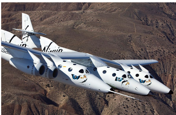
FIGURE 1. SpaceShipTwo carried aloft (in the center) under White Knight 2. Note the similarity of the cockpit and forward fuselage design. Courtesy of Scaled Composites/Virgin Galactic.
