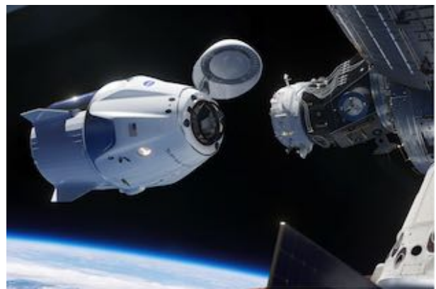
FIGURE 6. Artist's CAD rendering of a Crew Dragon approaching the docking port on the ISS. Courtesy of SpaceX.
