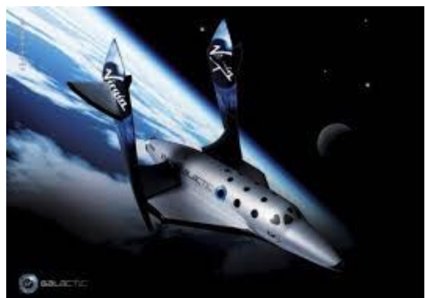
FIGURE 3. SpaceShipTwo with its wings in "feathered" position to commence its descent and re-entry. Courtesy of Scaled Composites/Virgin Galactic.
