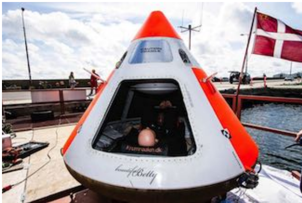
FIGURE 28. Advanced concept mock-up for the Copenhagen Suborbitals "Beautiful Betty" single person capsule, resembling a mini-Apollo capsule. Courtesy of Copenhagen Suborbitals.
