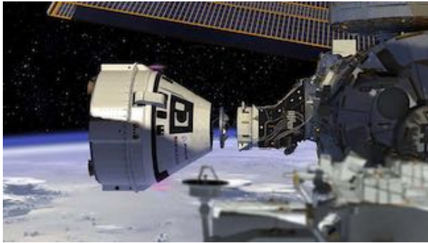
FIGURE 21. Boeing Starliner approaching the ISS to dock at the -V-Bar docking port on the Unity node. Note the extensible, impact absorbing docking collar. Courtesy of Boeing.
