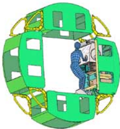
Figure 3. Four Stand-off rack arrangement of a “baloney slice” through an ISS module. The standoffs are the yellow arc segments at the corners. Credit: NASA.
