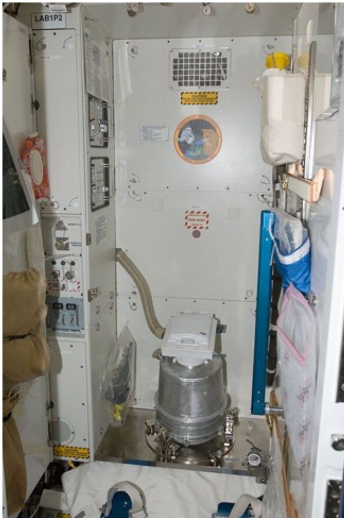
Figure 9. The Waste and Hygiene Compartment with space toilet in Node 3 Tranquility. NASA photo.
