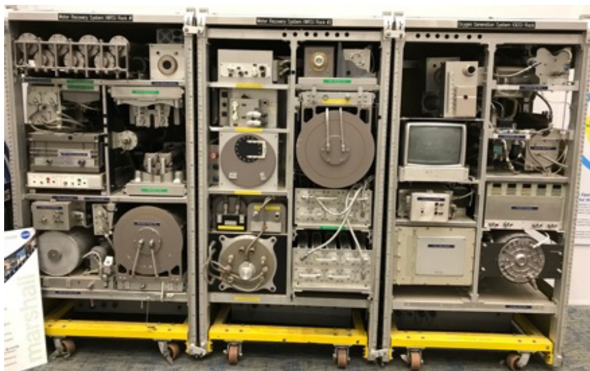
Figure 1. US ISS ECLSS Racks at NASA MSFC from the left: test racks versions of Water Processing, Urine Processing, and O 2 generation racks in ISS Node 3 Tranquility. Credit: NASA MSFC.
