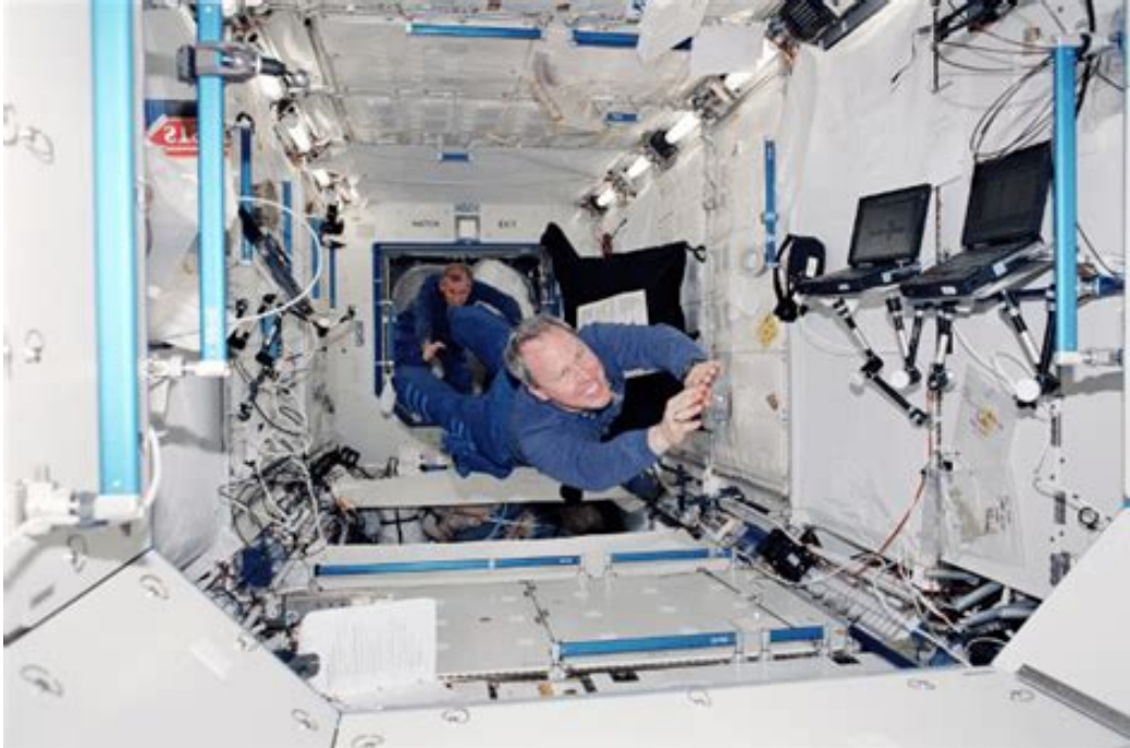
Figure 5. The US Destiny Lab early in its utilization on the ISS. Most of the rack faces exposed with blank cover panels. Credit: NASA.
