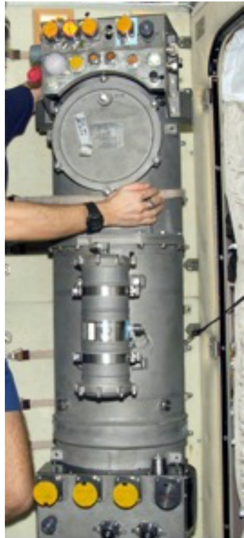
Figure 8. Russian Elektron O 2 Generator in the Zvezda Service Module. Courtesy of James Oberg.
