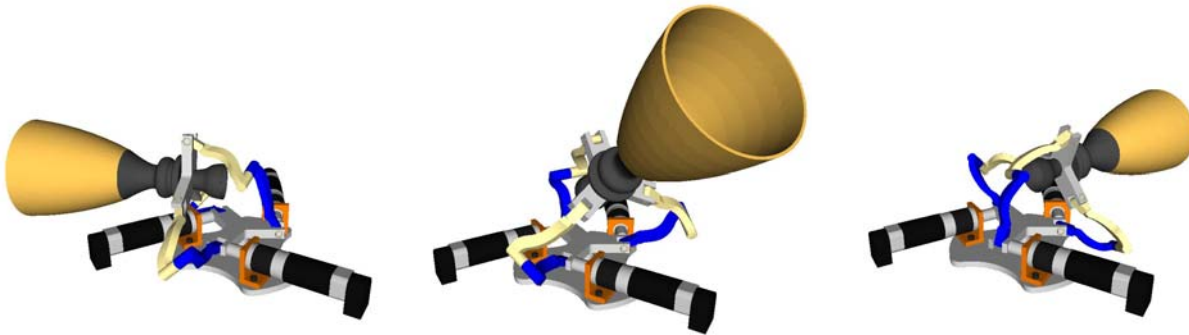
Figure 12: A series of still pictures showing a typical reaction-control thruster mounted on a Canfield joint, capable of pointing any direction within a hemisphere.
