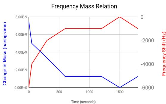
**Figure 4. The inverse relationship between the change in mass and the frequency shift.**
