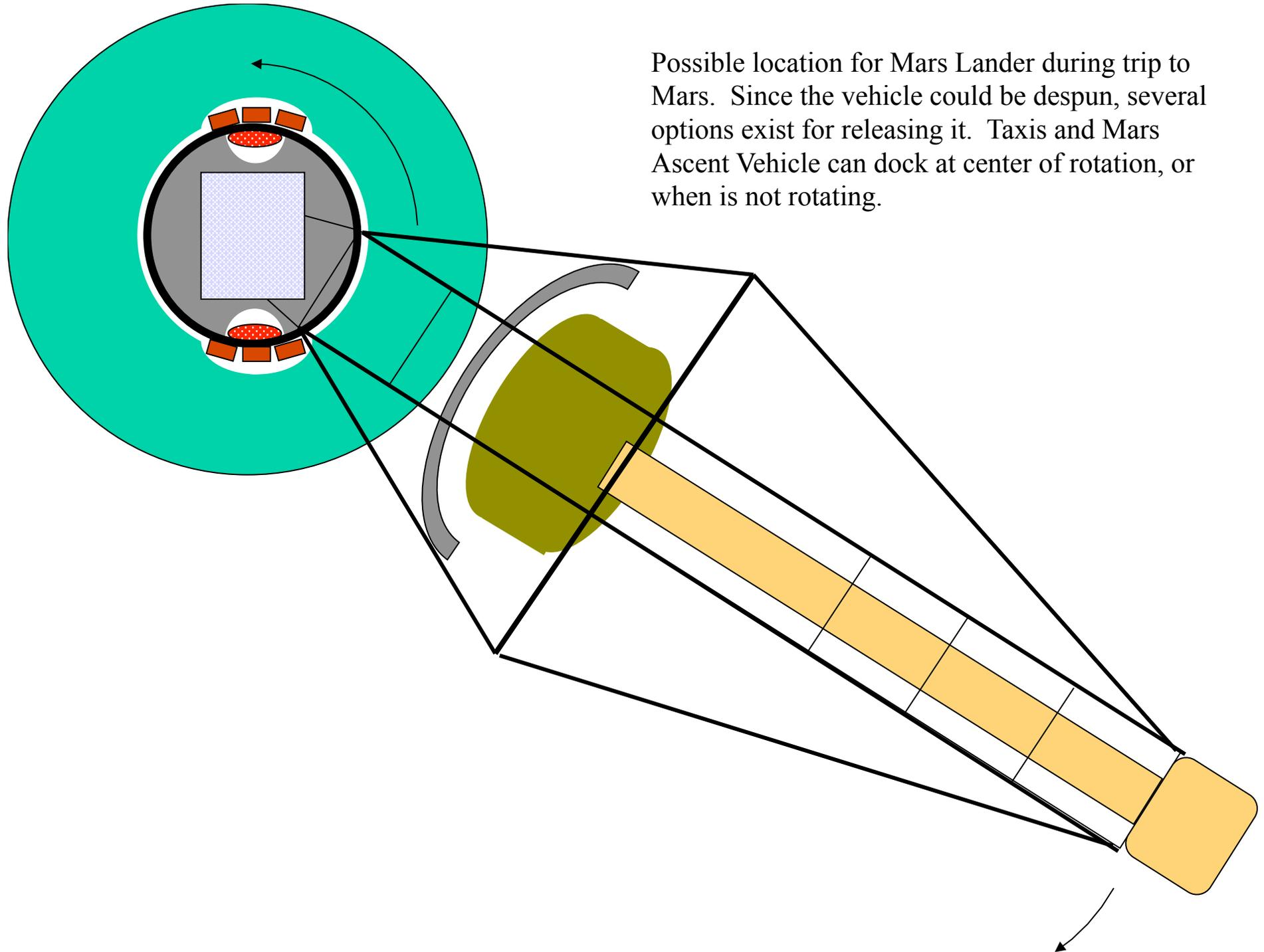
Possible location for Mars Lander during trip to Mars. Since the vehicle could be despun, several options exist for releasing it. Taxis and Mars Ascent Vehicle can dock at center of rotation, or when is not rotating.
