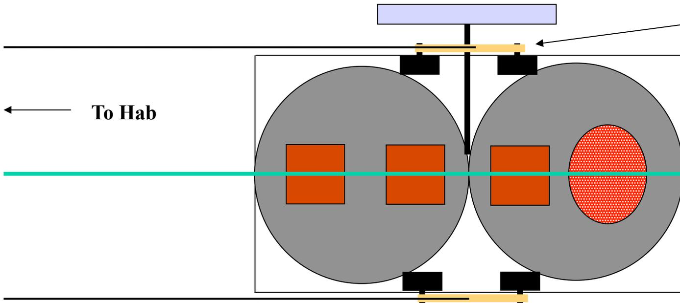
Planetary gear drive to allow prop and power to pass through center without moving joints. Makes it harder to replace tanks for new mission, but they could be refilled.
