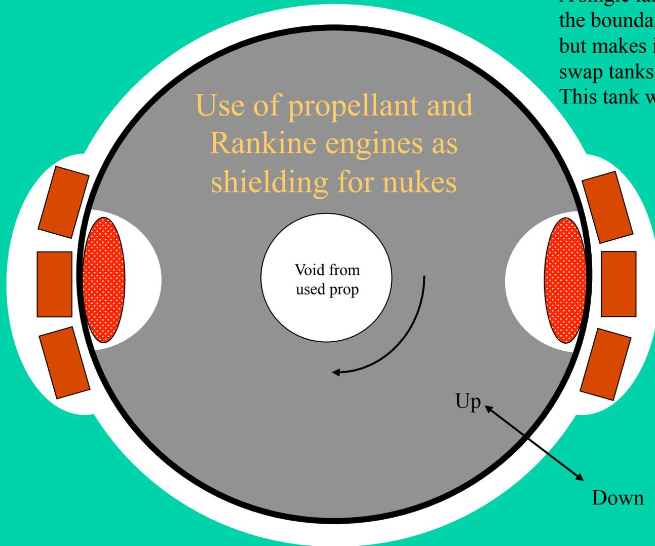
Single cylindrical propellant tank has squirrel cage track around its end caps. Recessed volumes carved out of tank for reactor. Rankine engines placed 'below' nuke, but vapor piped out of top of reactors to use natural boiling action to advantage. Pressure drop takes vapor to Rankine engines. Fluid then flows downhill to radiators. Propellant and engines serve as radiation shielding.
