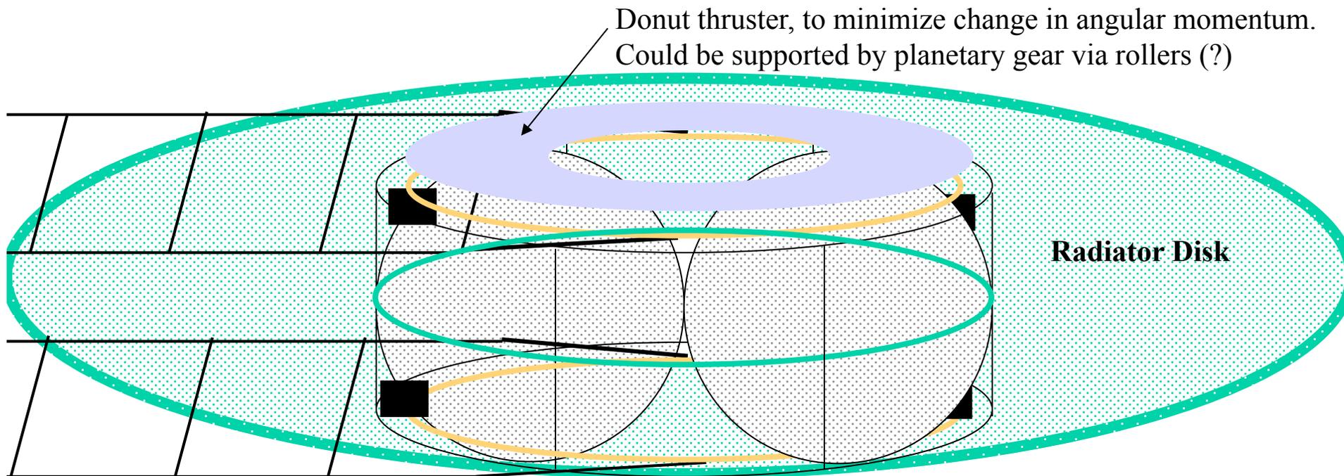
A single large tank defines the boundaries of the cage but makes it impossible to swap tanks for next flight. This tank would need to be refilled.
