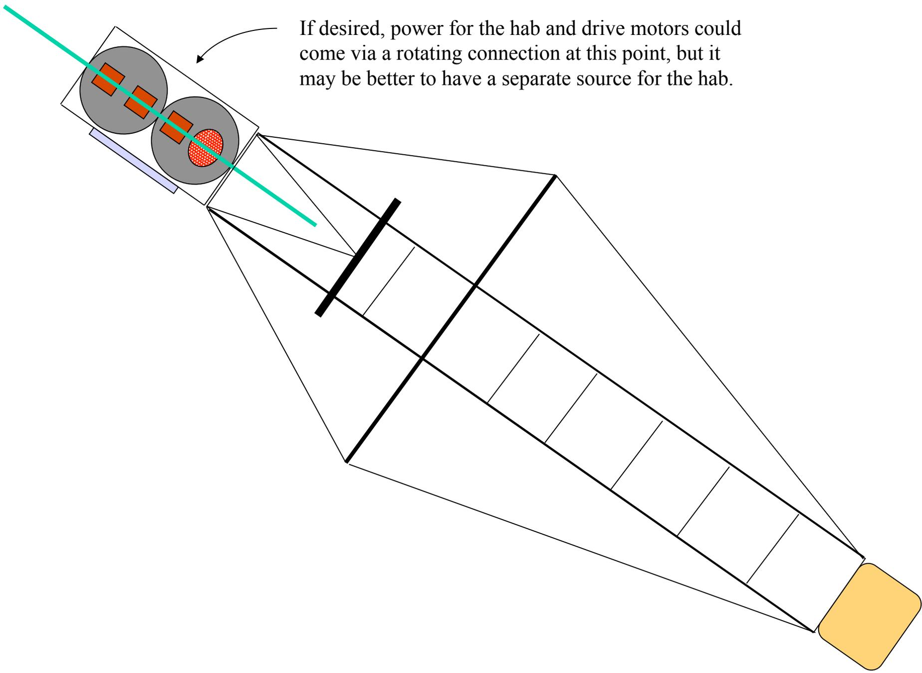
If desired, power for the hab and drive motors could come via a rotating connection at this point, but it may be better to have a separate source for the hab.
