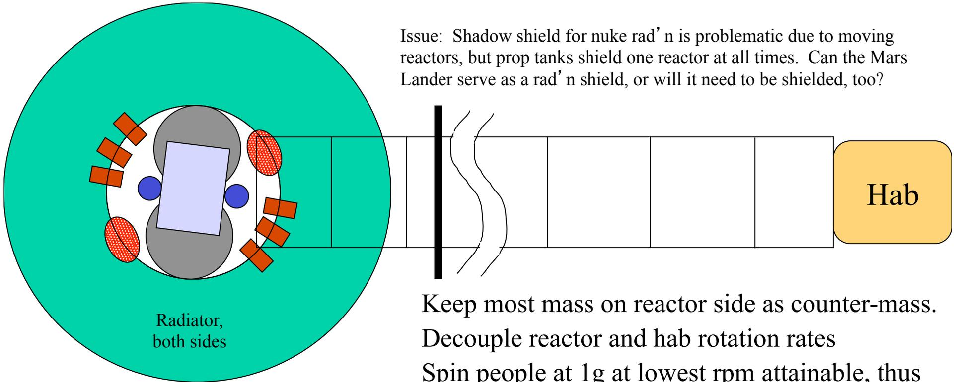
Keep most mass on reactor side as counter-mass.
