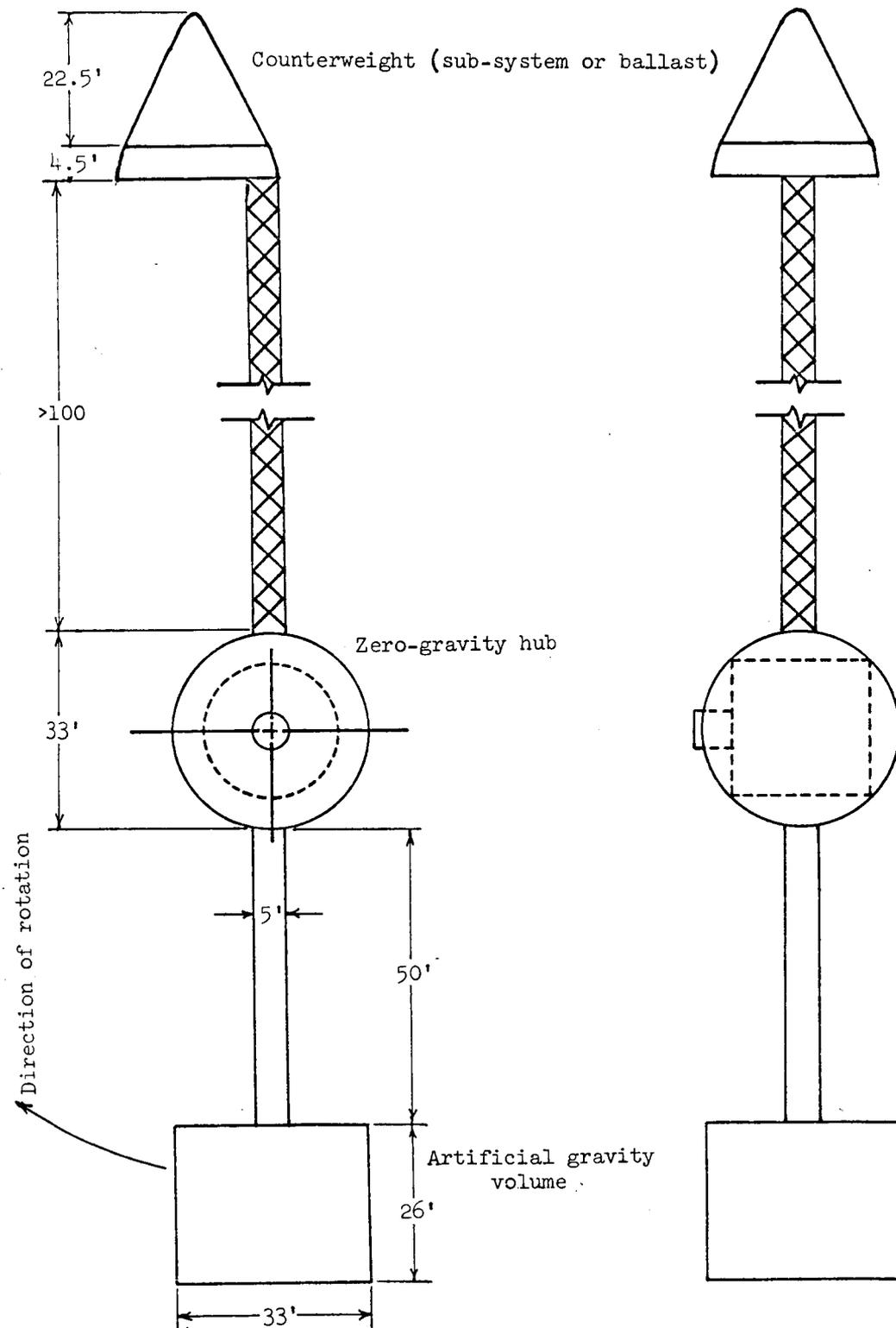
Figure 1-1 - Configuration no. 1, dumbbell space station, deployed.
