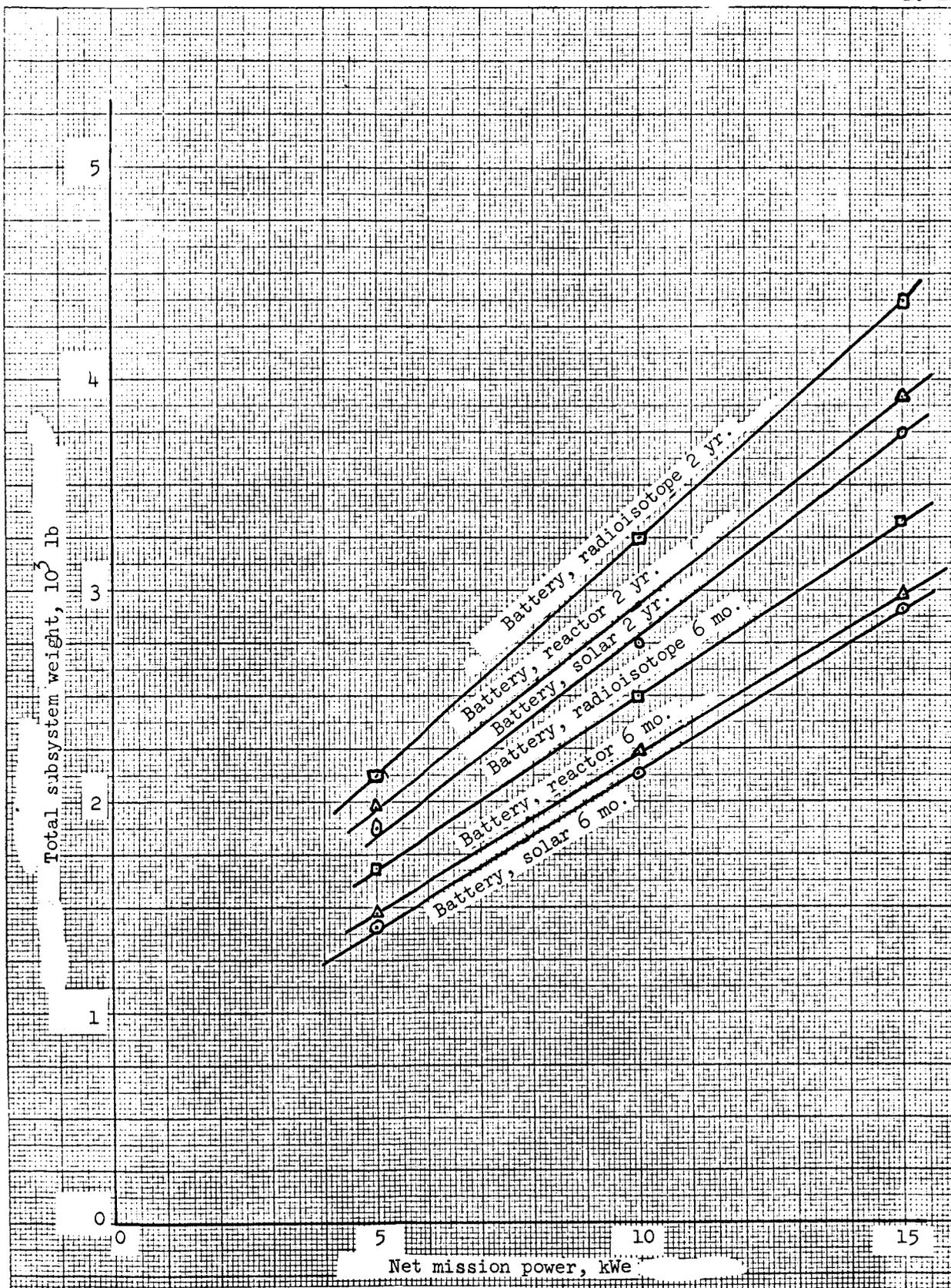
Figure 1.26 - Low Earth orbit battery supplementary power subsystems.
