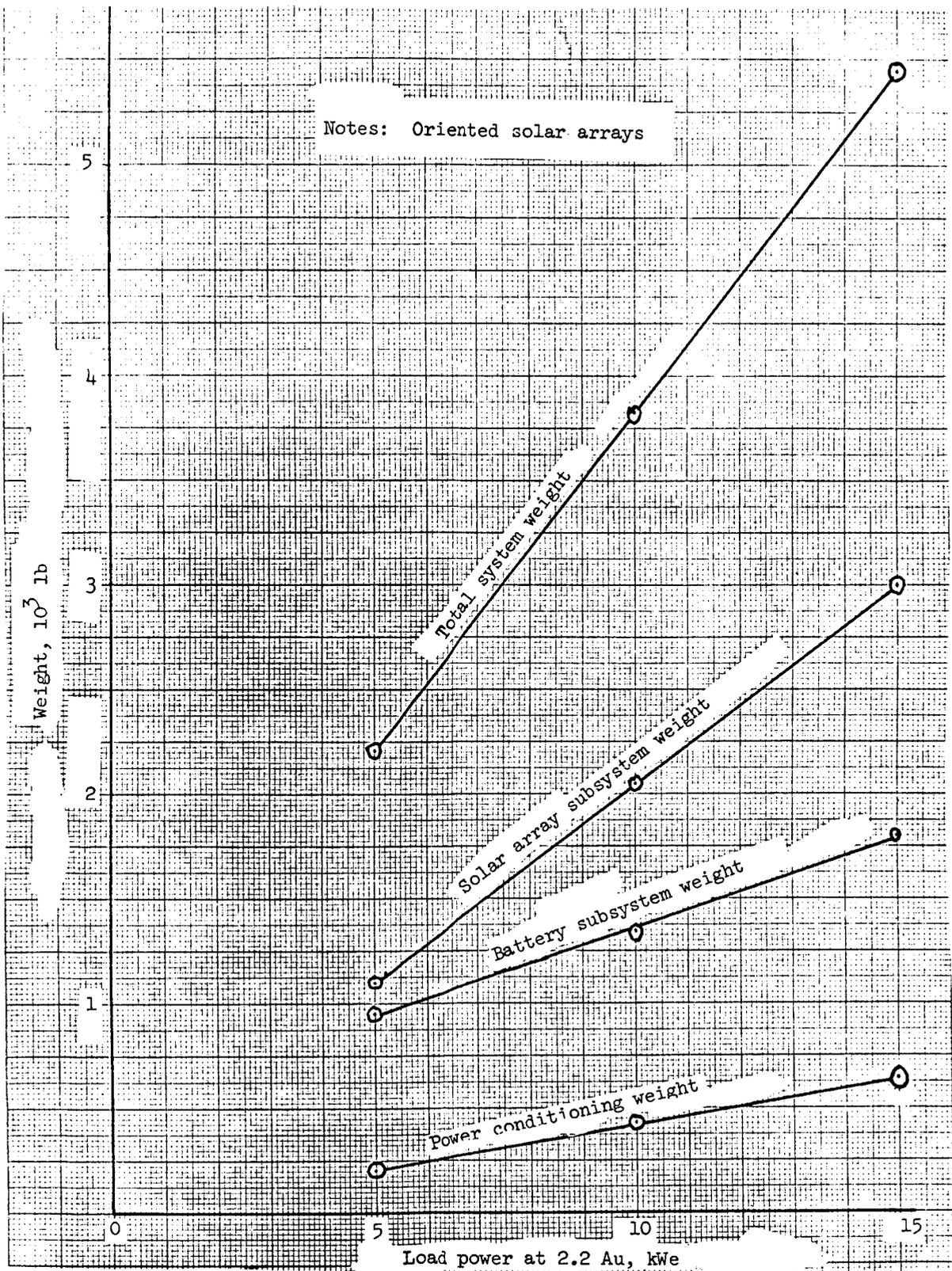
Figure 1.50 - Solar cell/battery system weight versus load power, Mars flyby.
