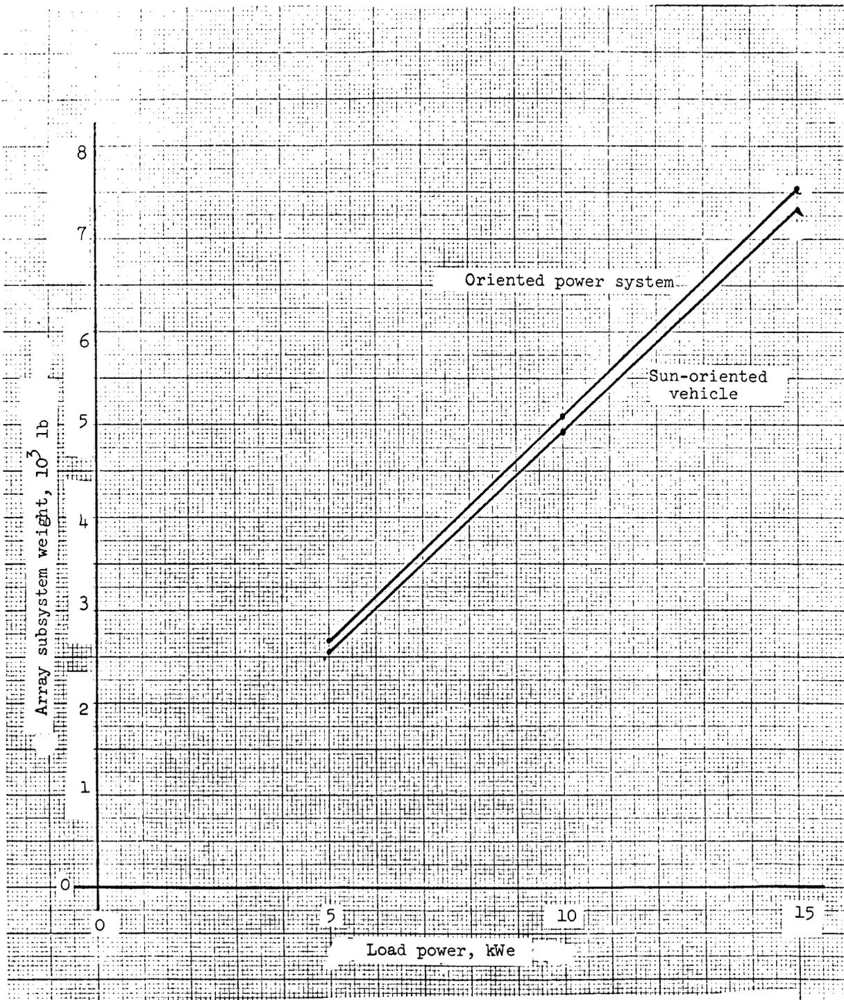
Figure 1.45 - Array subsystem weight versus load power, low Earth orbit missions.
