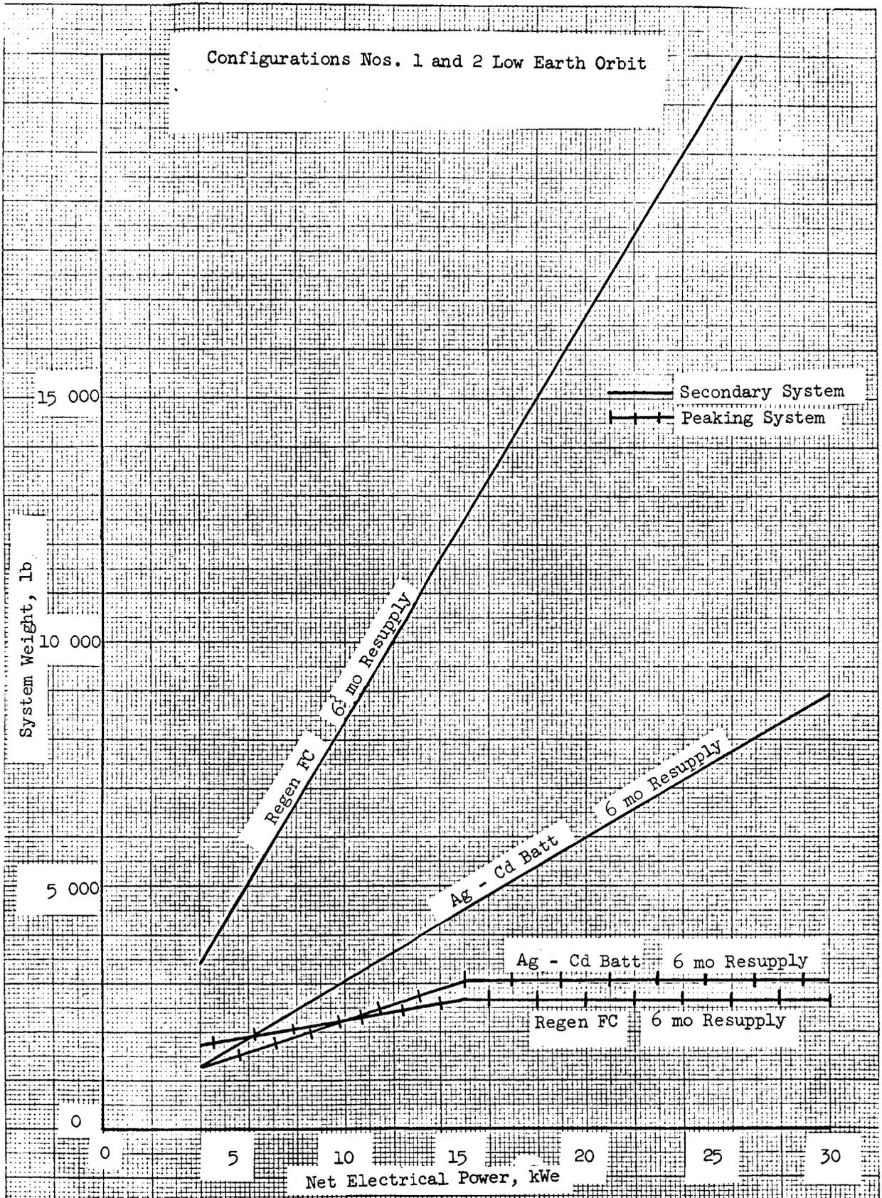
Figure 1.96 - Secondary power system weight versus net electrical power, LEO
