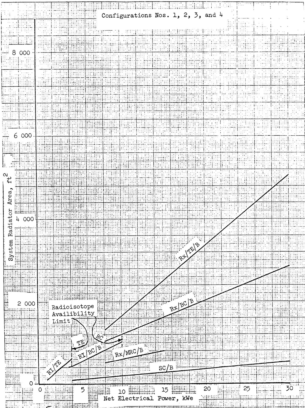
Figure 1.103- Power system radiator area versus net electrical power
