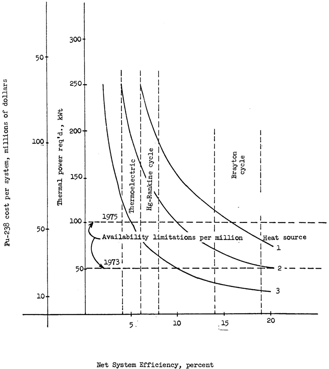
Figure 1.24 - Required thermal power and cost versus net system efficiency.
