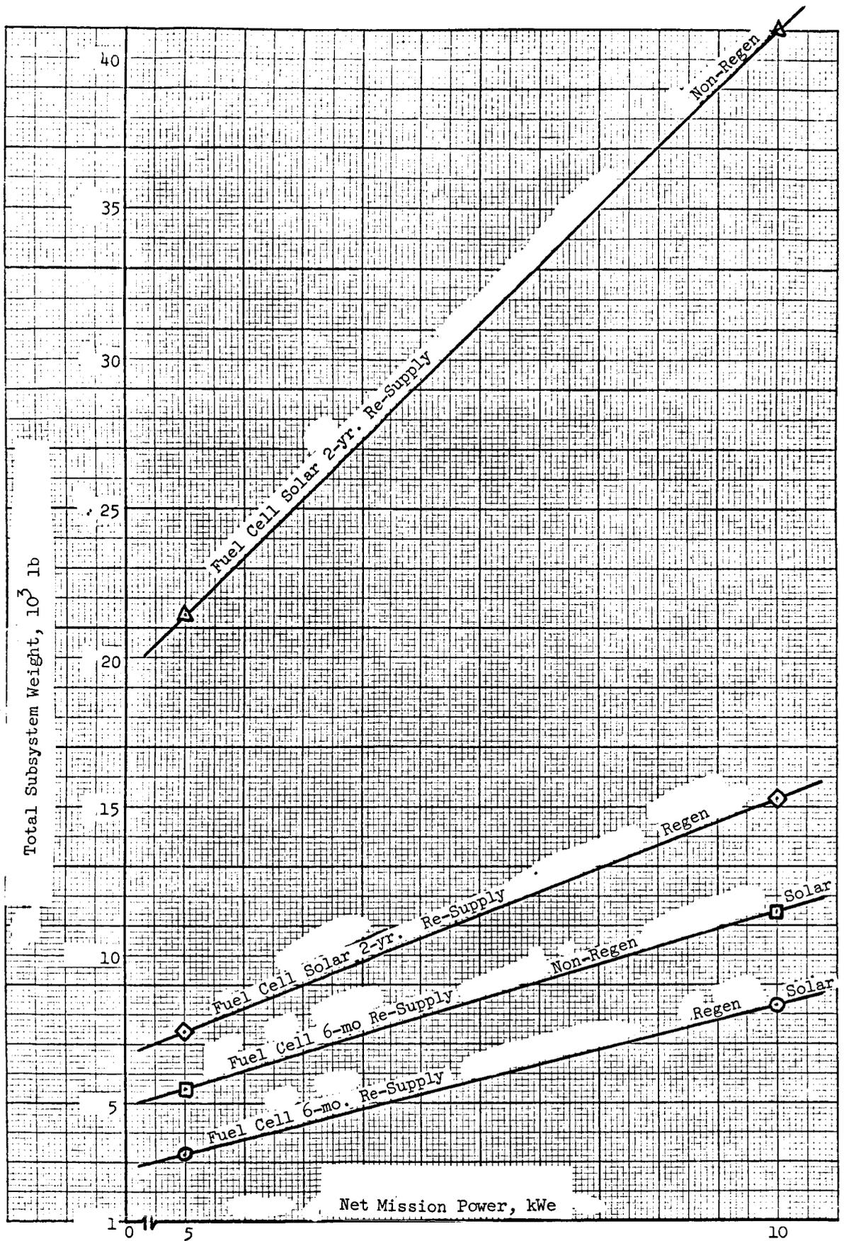
Figure 1.32 - Low Earth orbit fuel cell complementary power subsystems.
