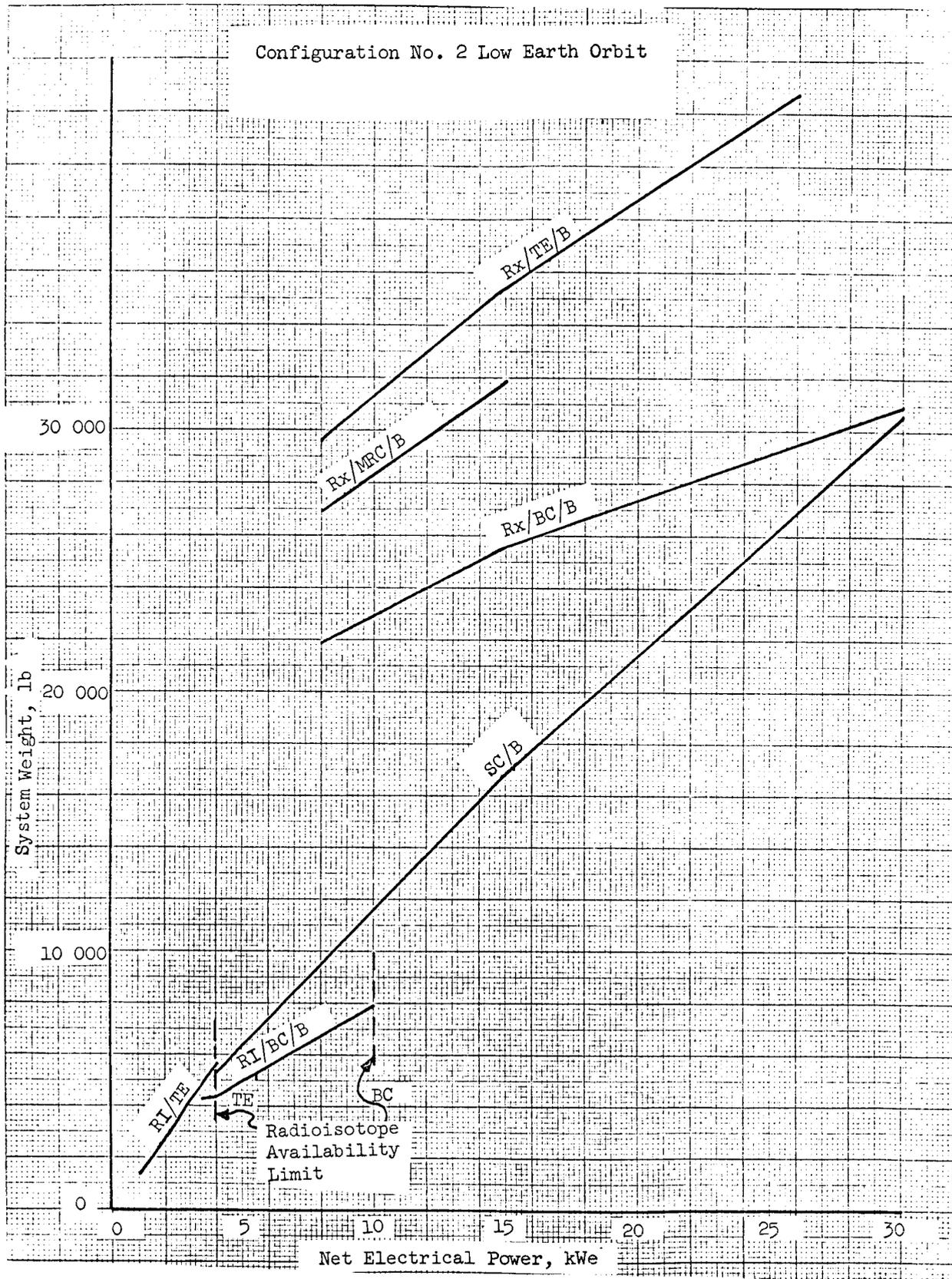
Figure 1.93 - Power system weight versus net electrical power, LEO no. 2
