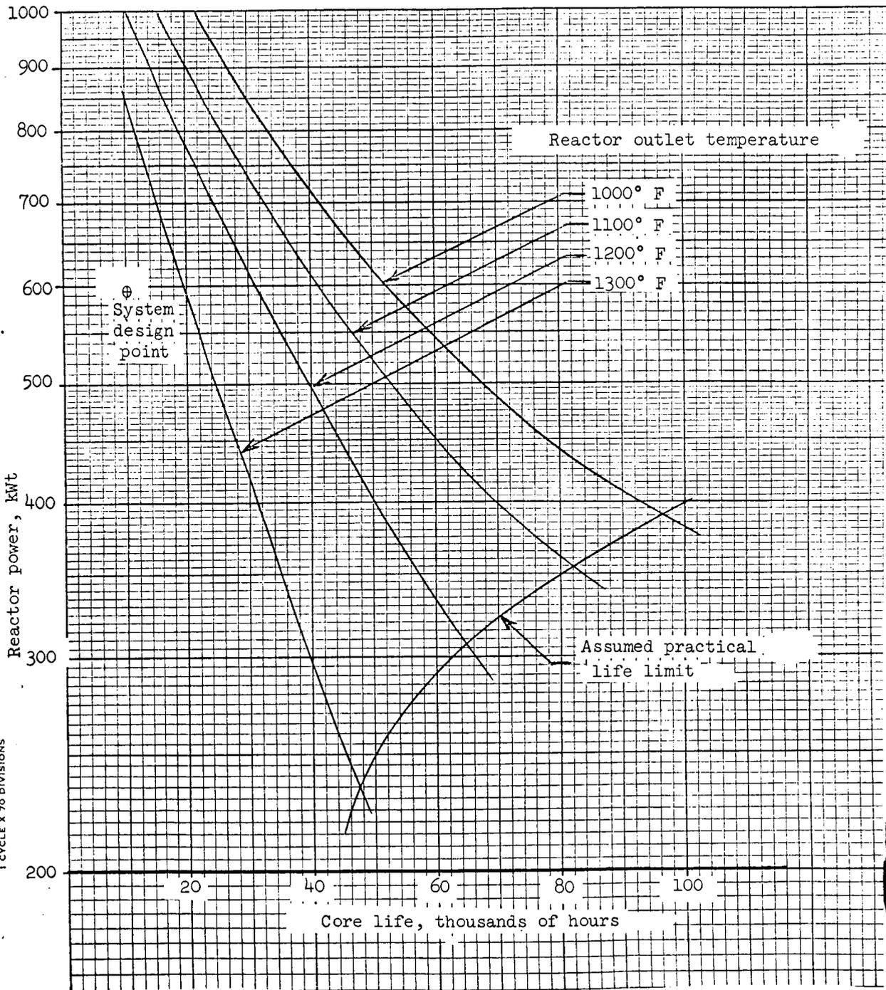
Figure 1.57 - SNAP-8 reactor operating capability.
