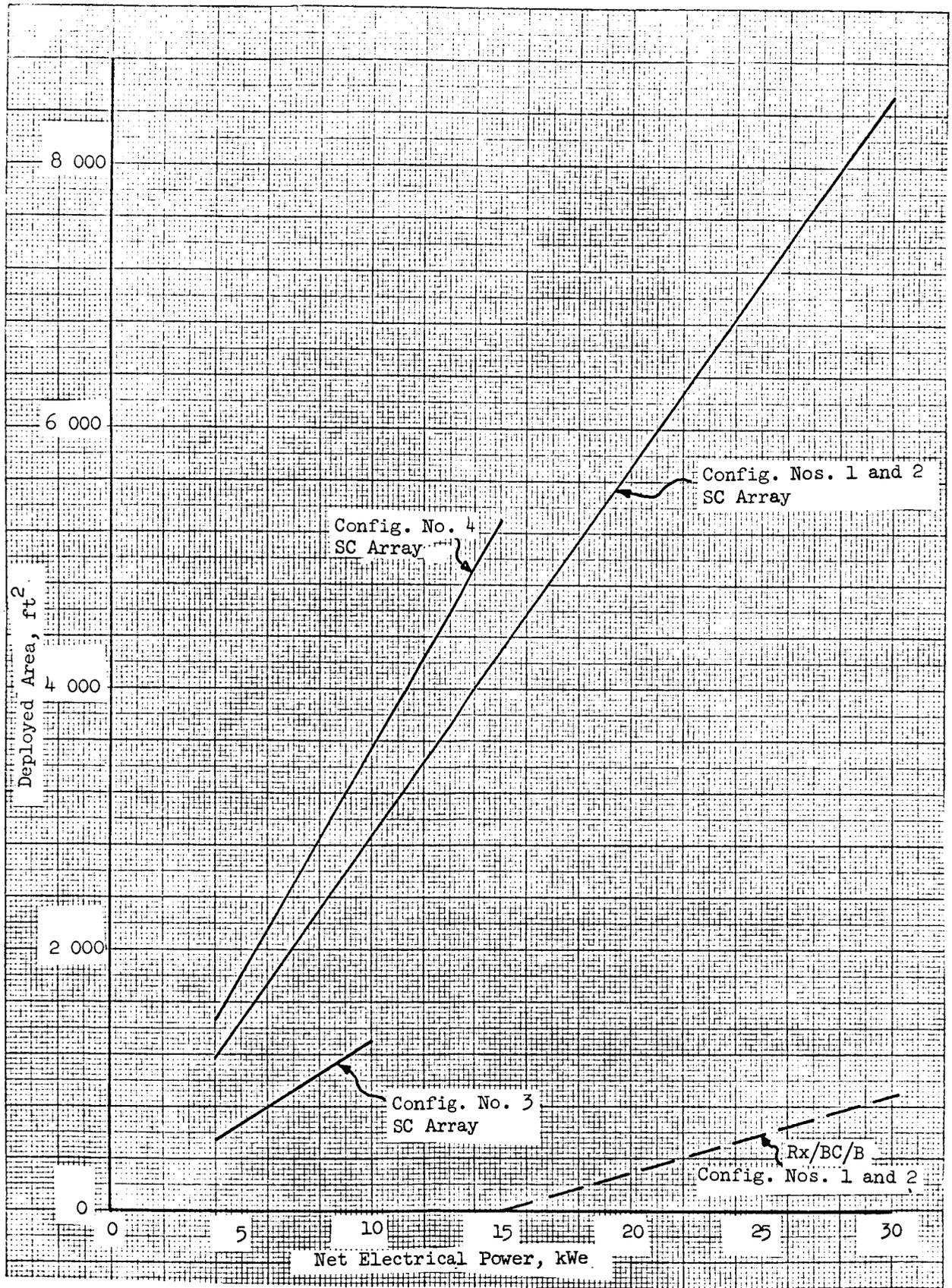
Figure 1.102- Power system deployed area versus net electrical power
