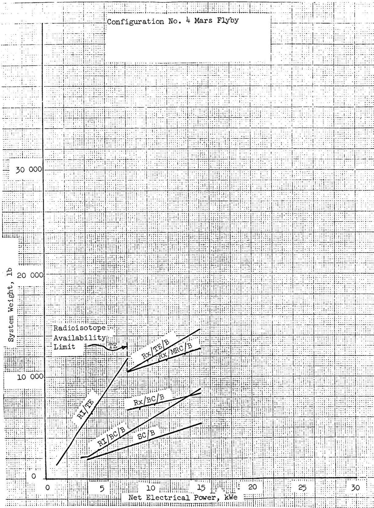
Figure 1.95 .- Power system weight versus net electrical power, Mars
