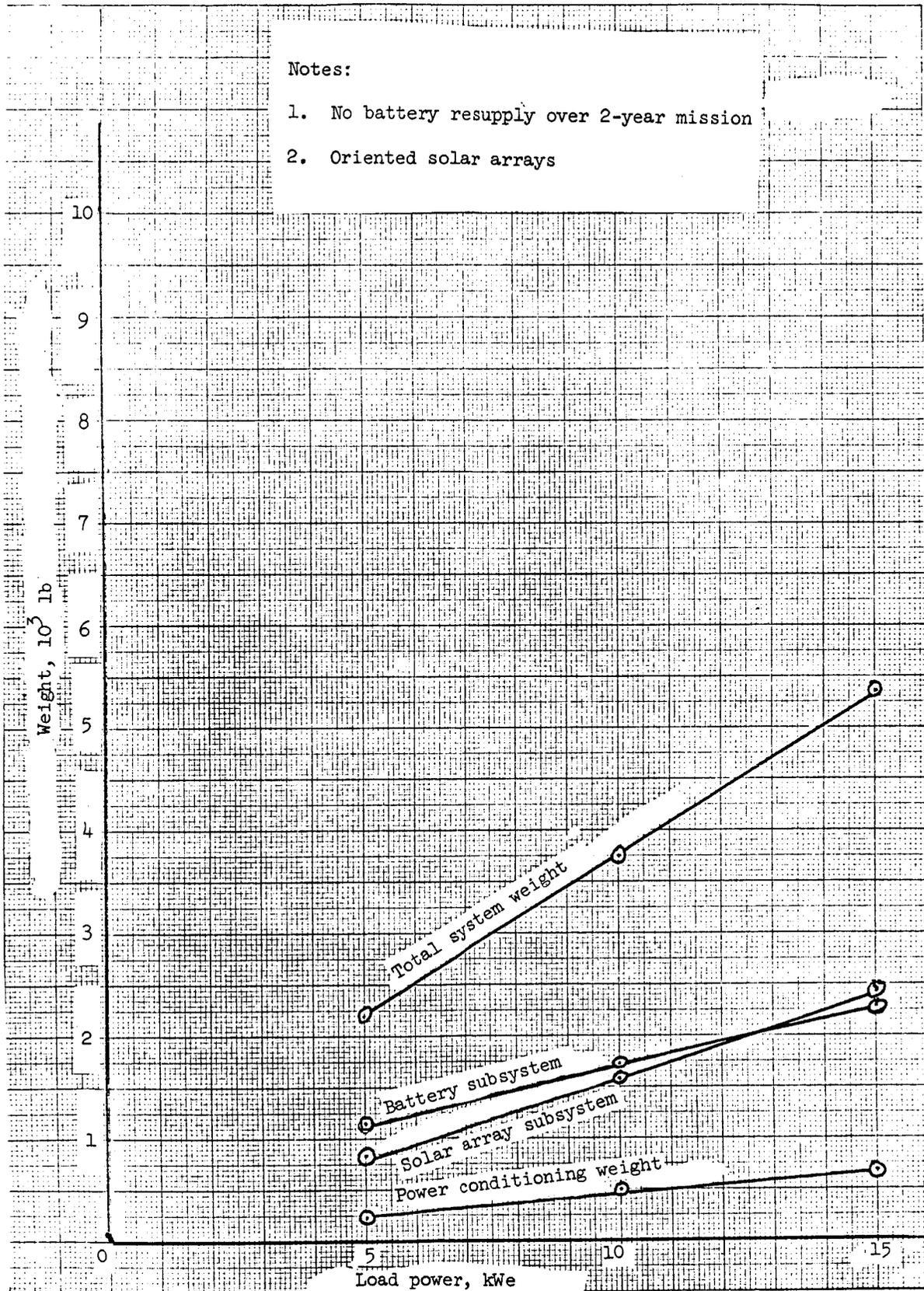
Figure 1.52 - Solar cell/battery system weight vs. load power, sync missions.
