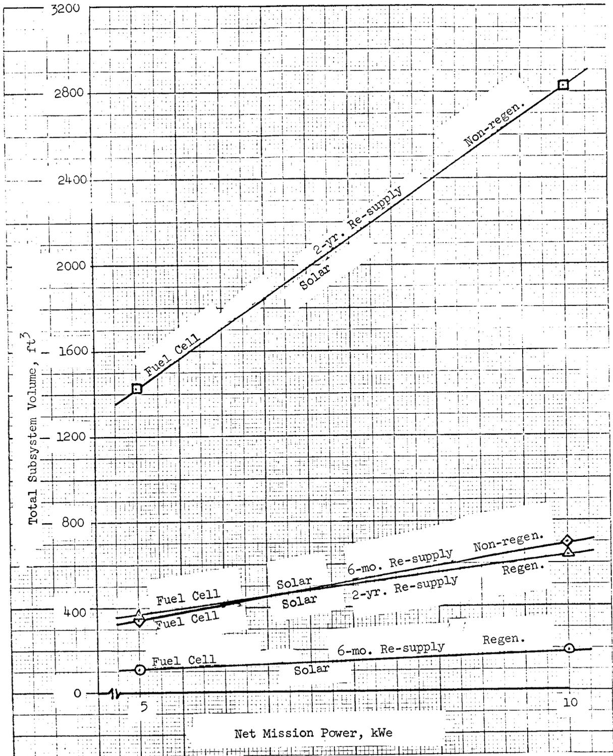
Figure 1.37 - Low Earth orbit fuel cell complementary power subsystems volume.
