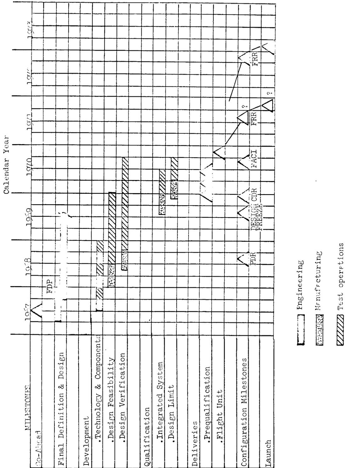
Figure 1.88 - Thermoelectric system development schedule, power sections.
