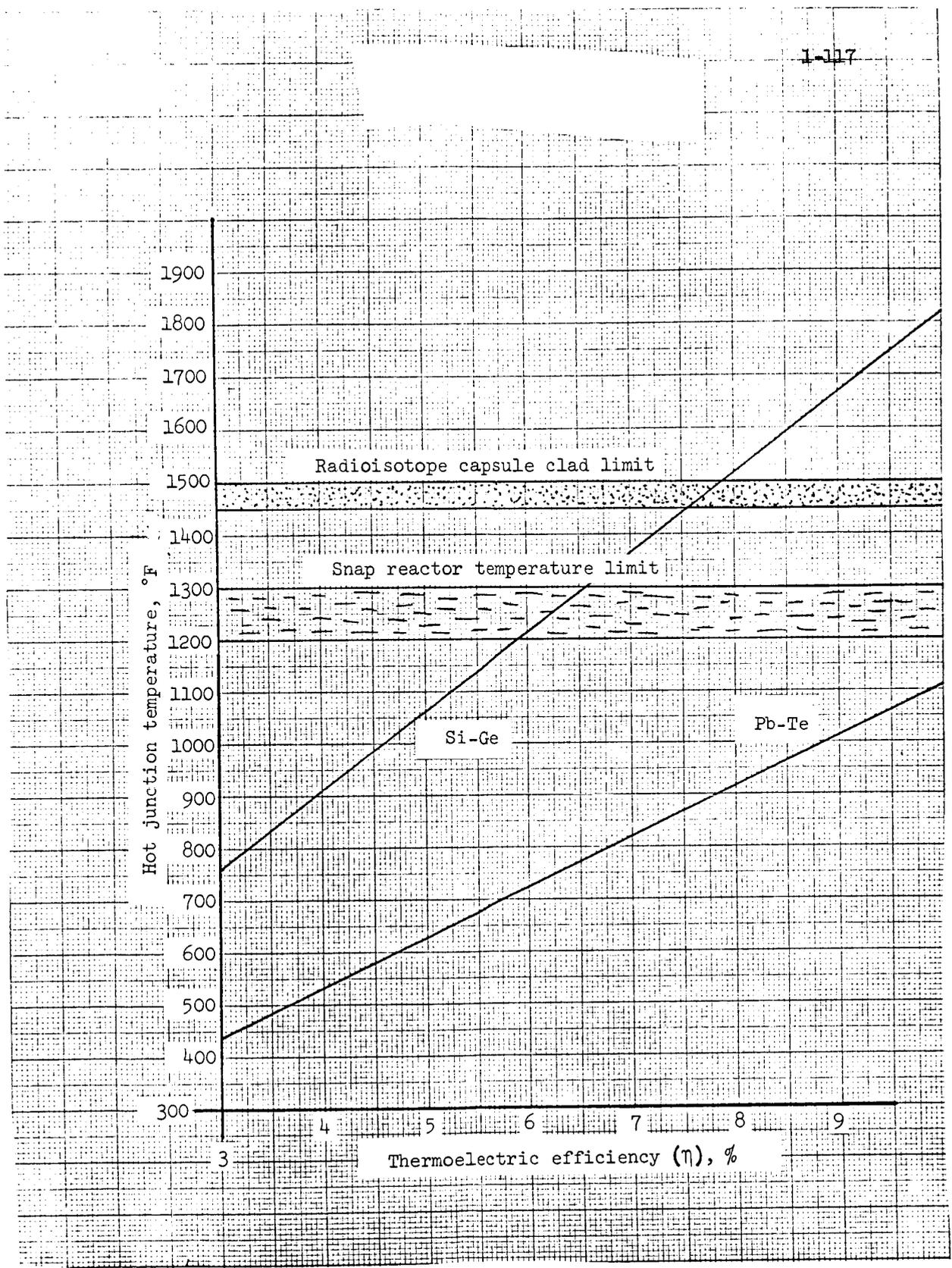
Figure 1.22 - Hot junction temperature versus thermoelectric efficiency.
