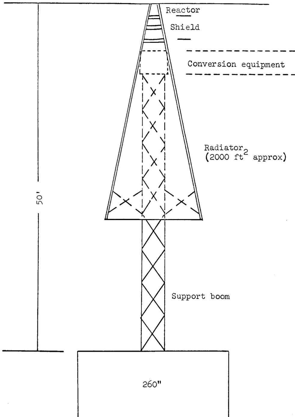
Figure 1.65 - Reactor thermoelectric system concept, Mars flyby.
