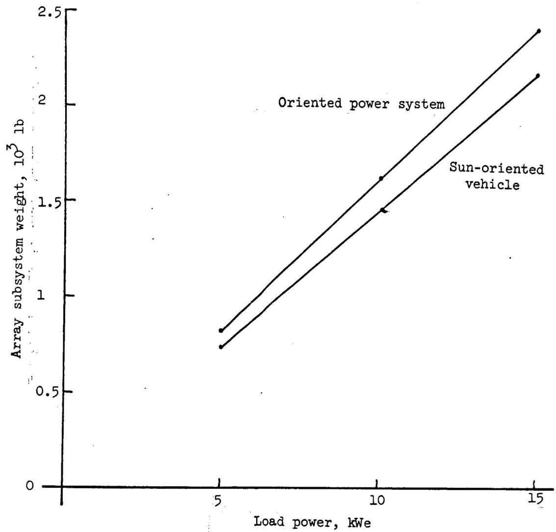
Figure 1.46 - Subsystem array weight versus load power, synchronous orbit missions.
