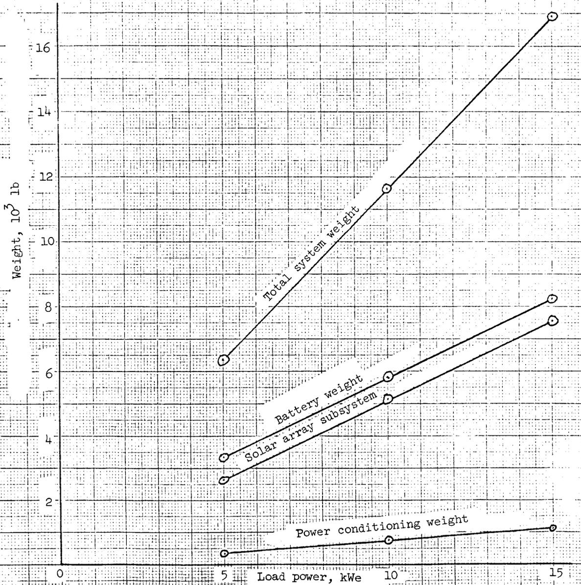
Figure 1.51 - Solar cell/battery system weight versus load power, LEO missions.
