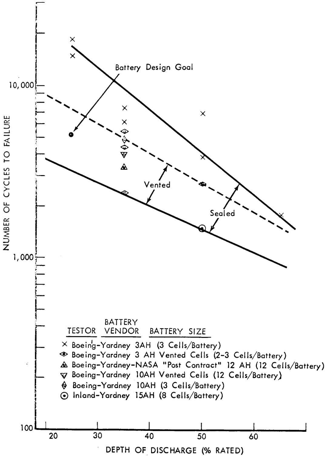
Figure 1.19 - Silver cadmium cell cycle life data.
