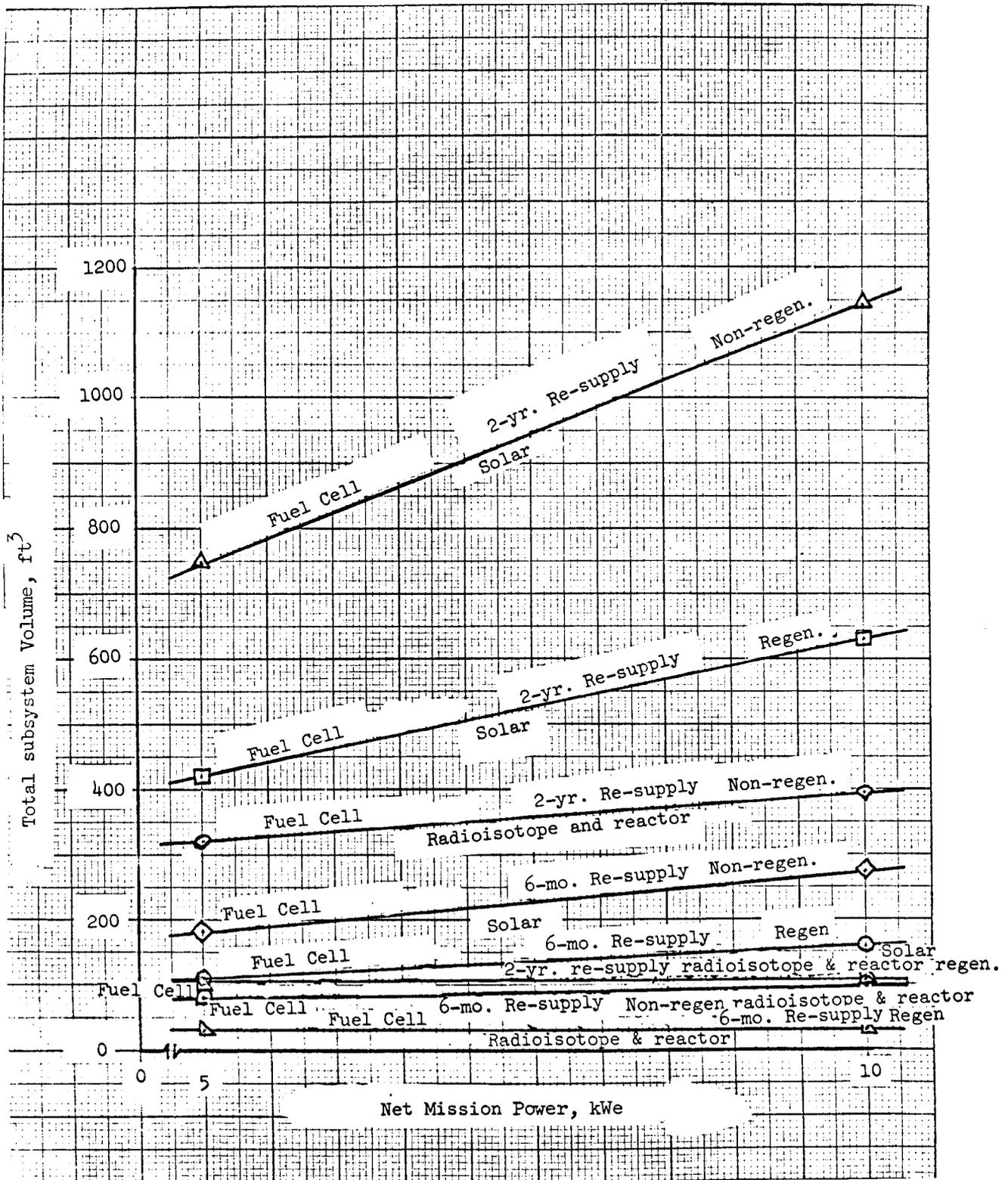
Figure 1.39 - Synchronous Earth orbit fuel cell supplementary power subsystems volume.
