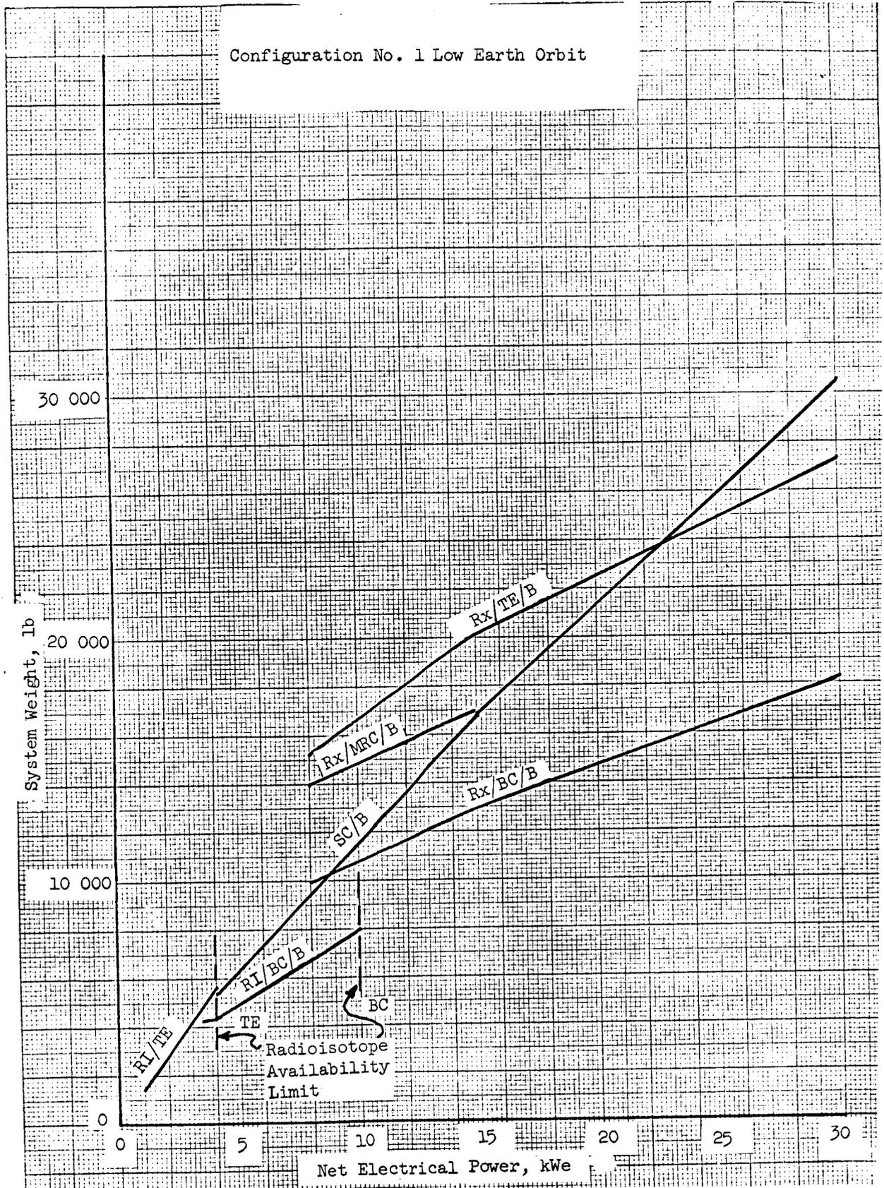
Figure 1.92 - Power system weight versus net electrical power, LEO no. 1
