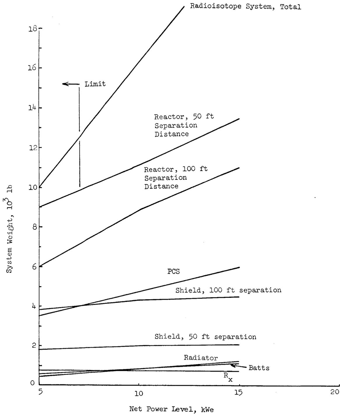
Figure 1.77 - Mars Flyby Mission: System weight vs net power level for radioisotope and reactor systems using mercury-Rankine.
