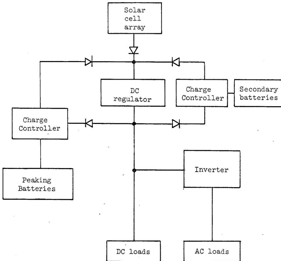
Figure 1.53 - LEO solar cell/battery schematic.
