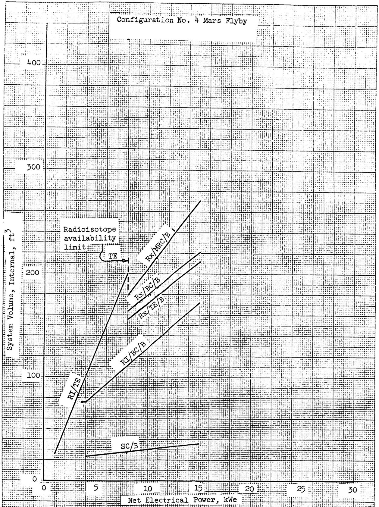
Figure 1.100- Power system volume versus net electrical power, Mars
