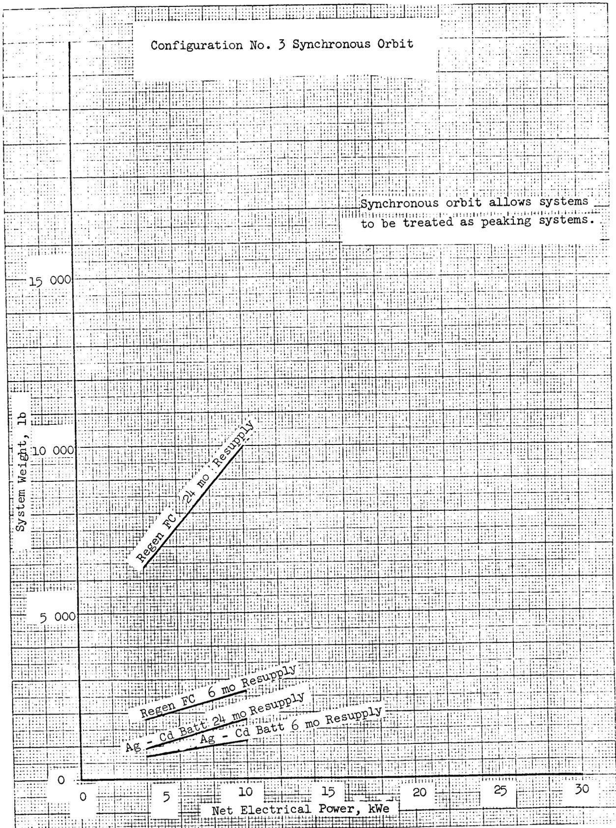
Figure 1.97 - Secondary power system weight versus net electrical power, sync
