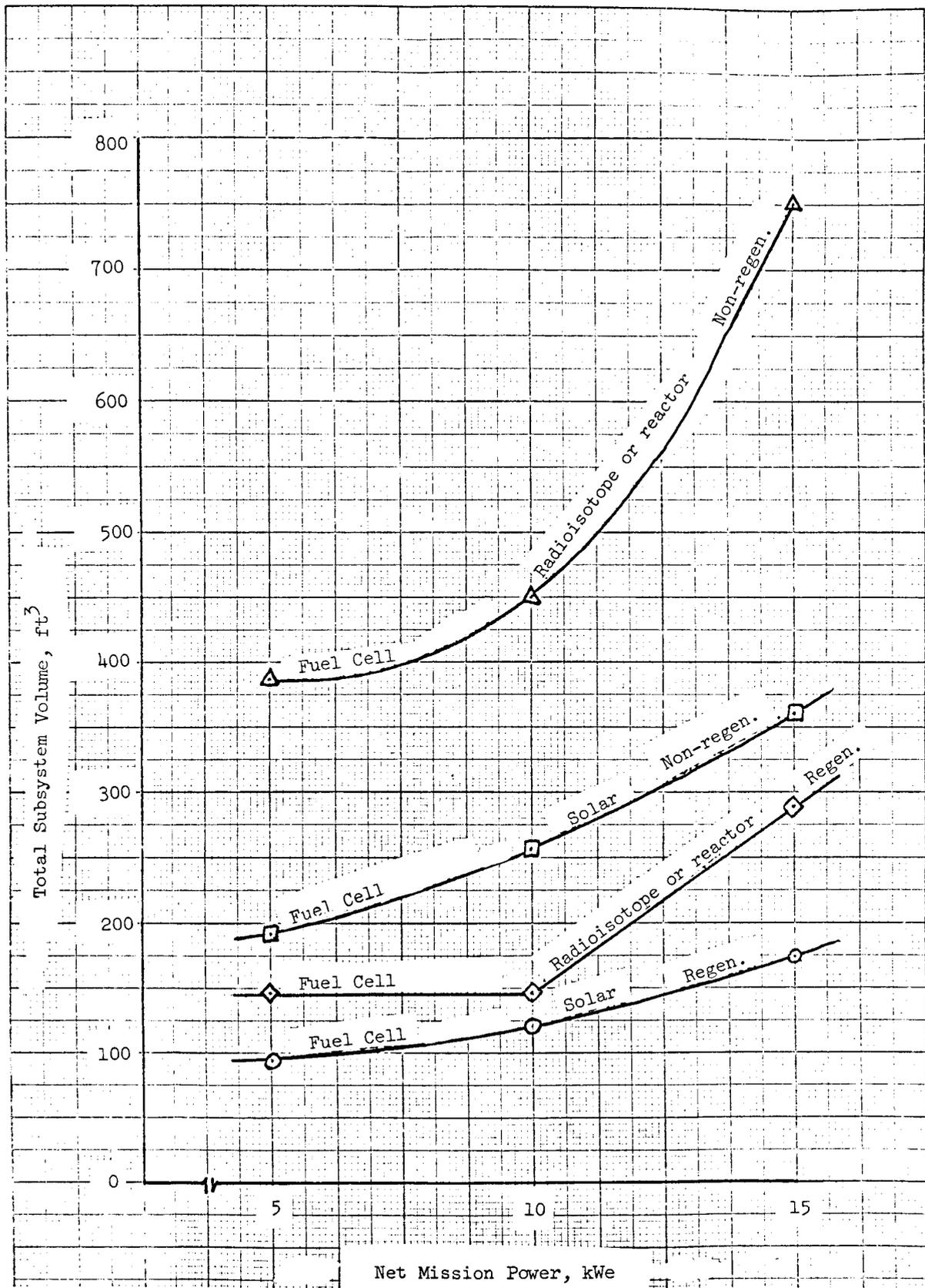
Figure 1.35 - Mars flyby fuel cell supplementary power subsystems volume.
