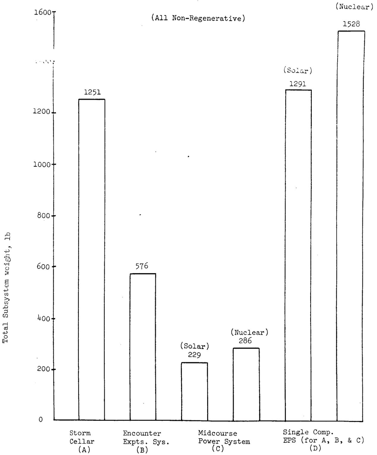
Figure 1.31 - Mars flyby fuel cell power subsystems.
