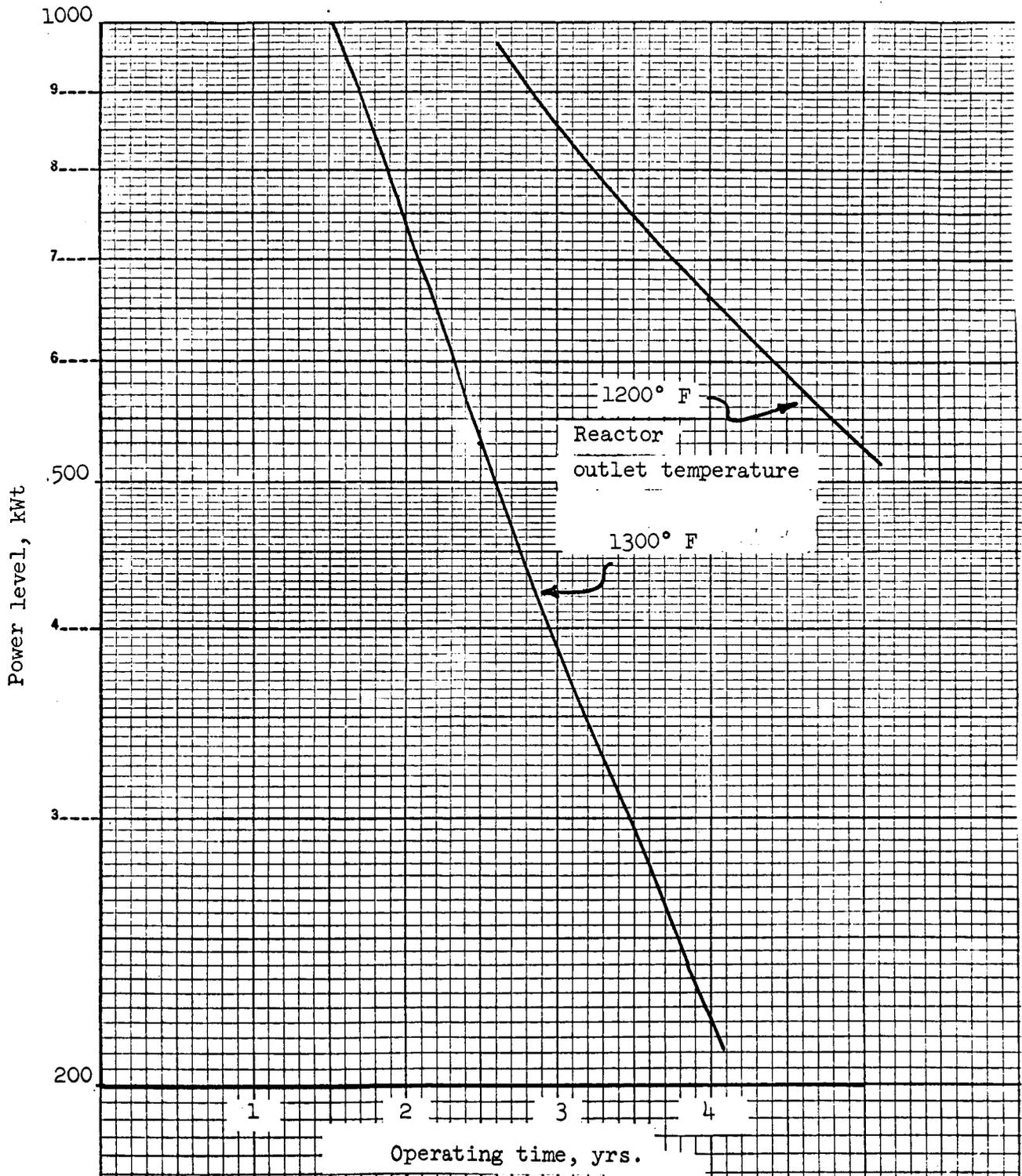
Figure 1.58 - Reactor operating characteristic (modified SNAP 8).
