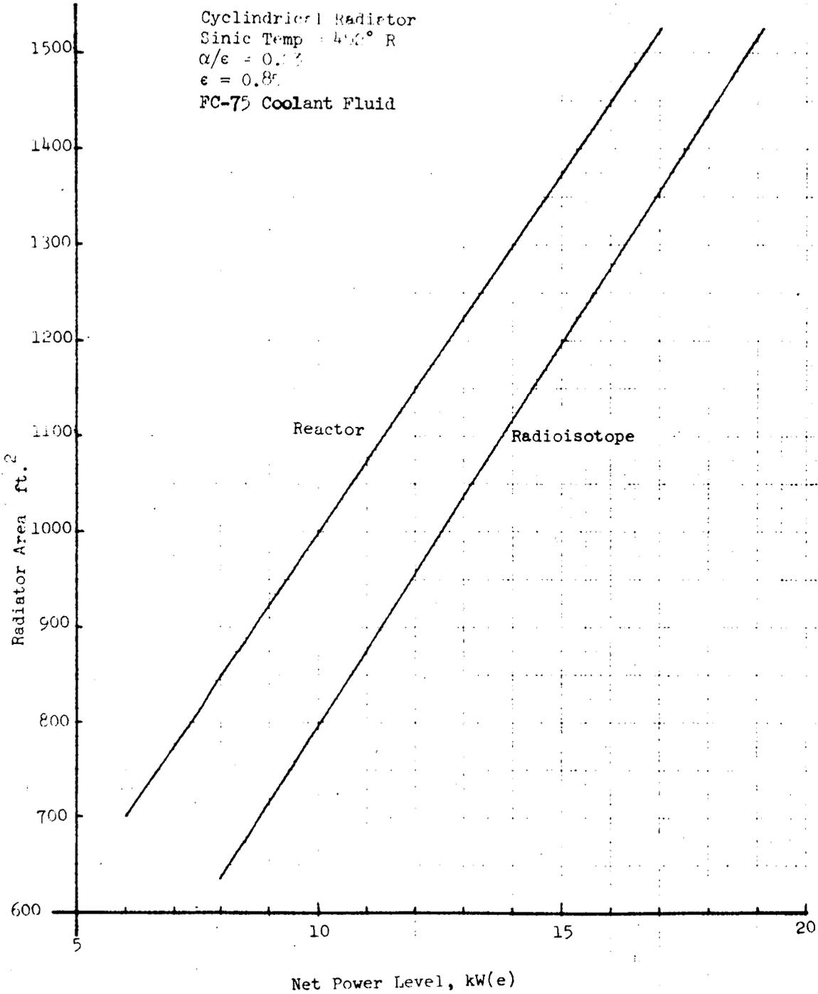
Figure 1-71 . - Radiator area required versus net power level for reactor and radioisotope Brayton-cycle systems.
