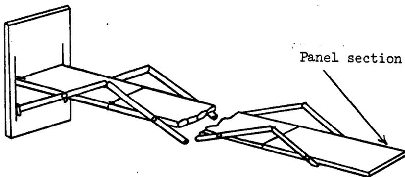
Figure 1.42 . - Concept "A" - rigid panel deployment concept.
