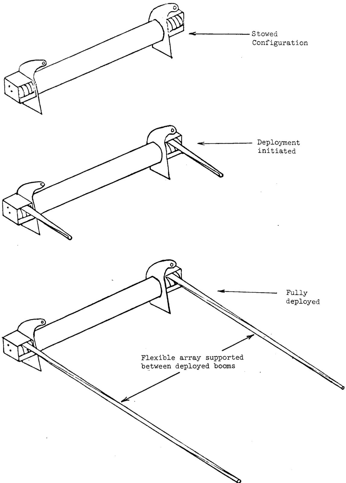
Figure 1.43 - Concept "B" - unfurlable array deployment concept.
