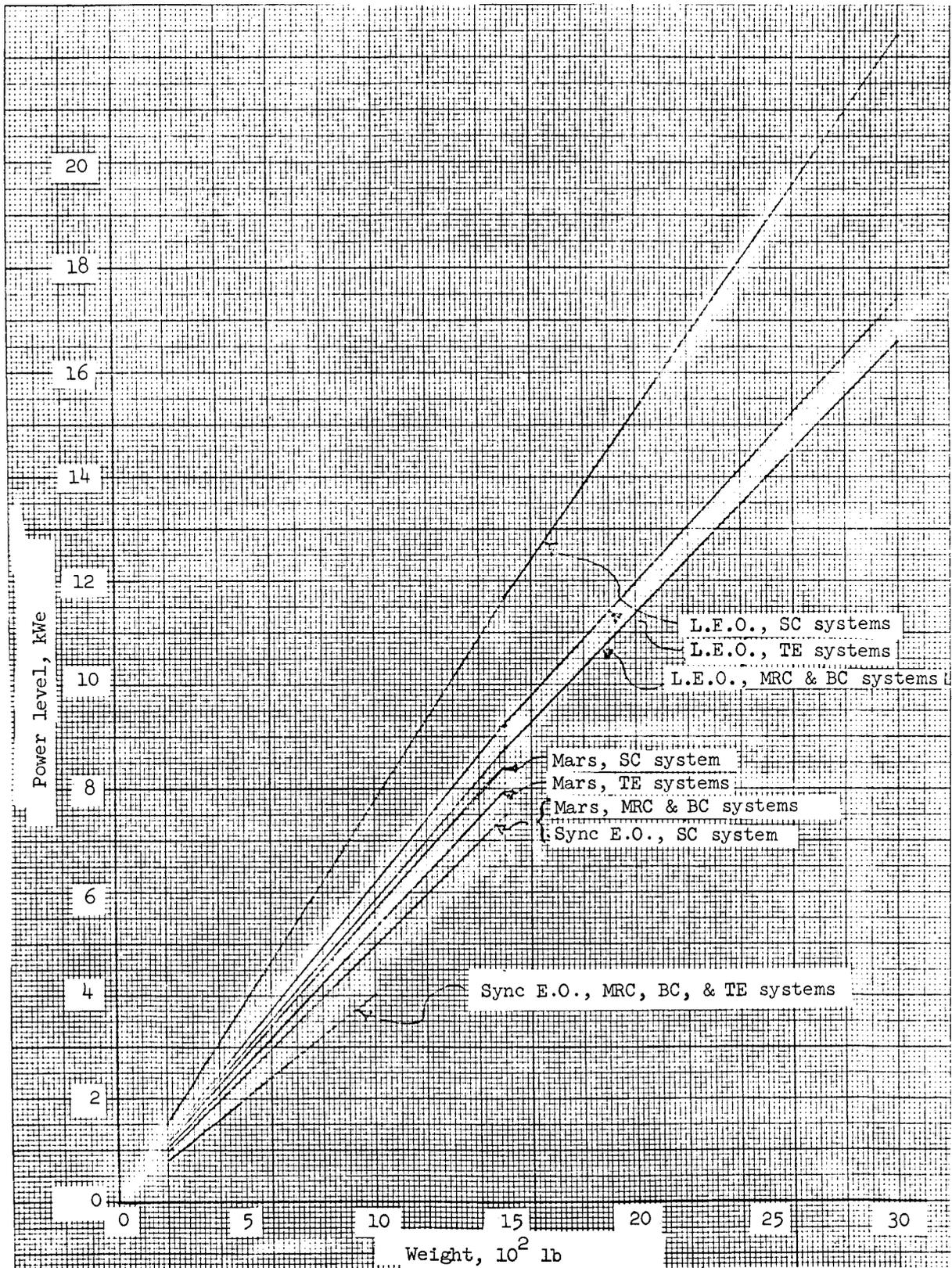
Figure 1.41 - Power conditioning weights vs power level.
