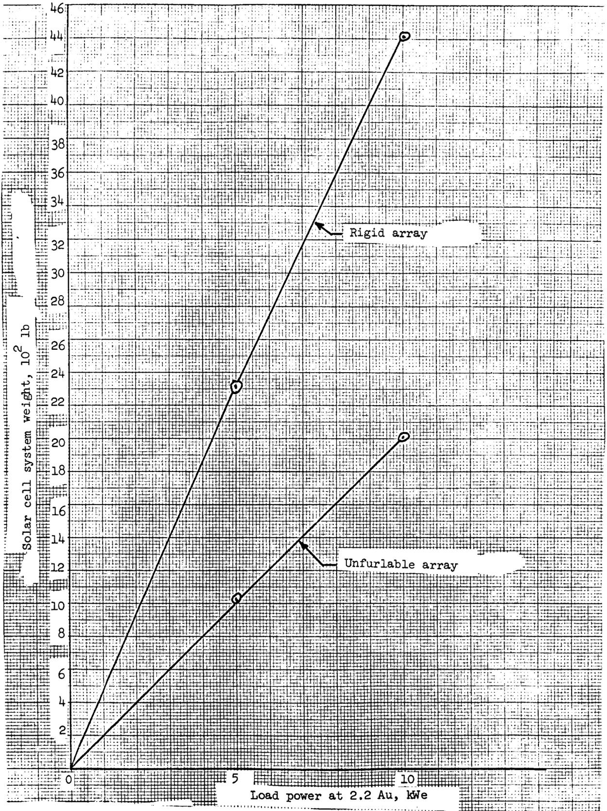
Figure 1.49. - Mars flyby solar cell system weight versus power.
