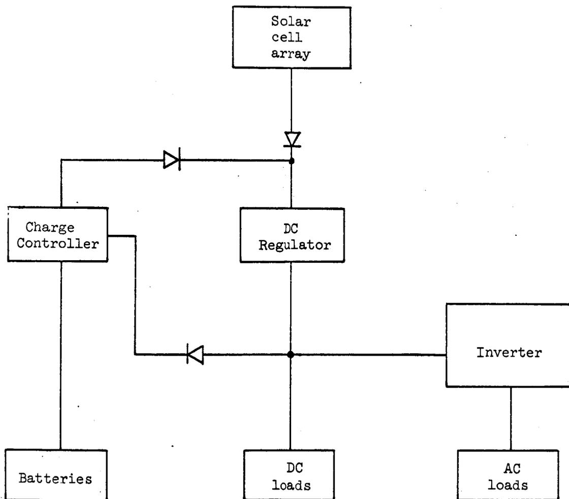
Figure 1.54 - Mars and sync solar cell/battery schematic.
