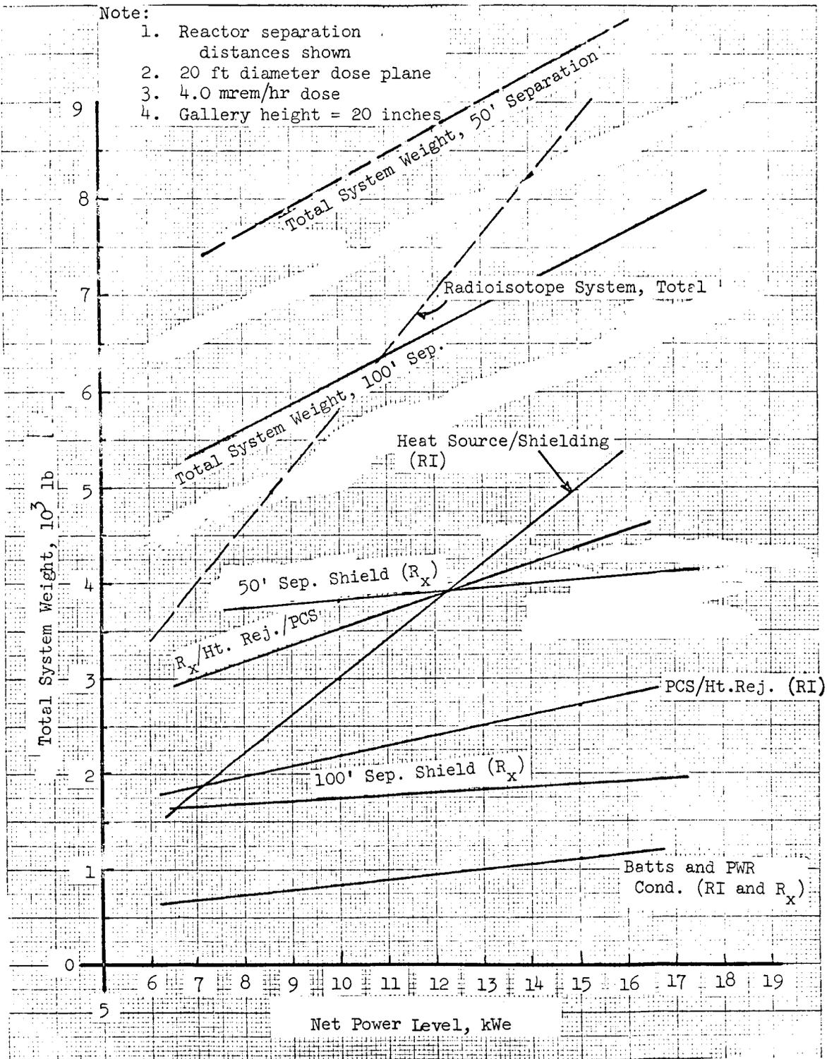
Figure 1.73 - Mars Flyby Mission: Total system weight versus net power level for reactor and radioisotope Brayton-cycle systems.
