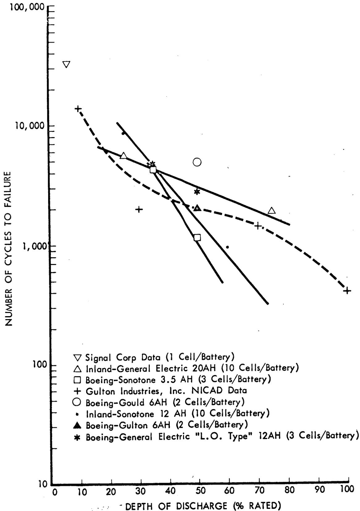
Figure 1.18 - Nickel cadmium cell cycle life data.
