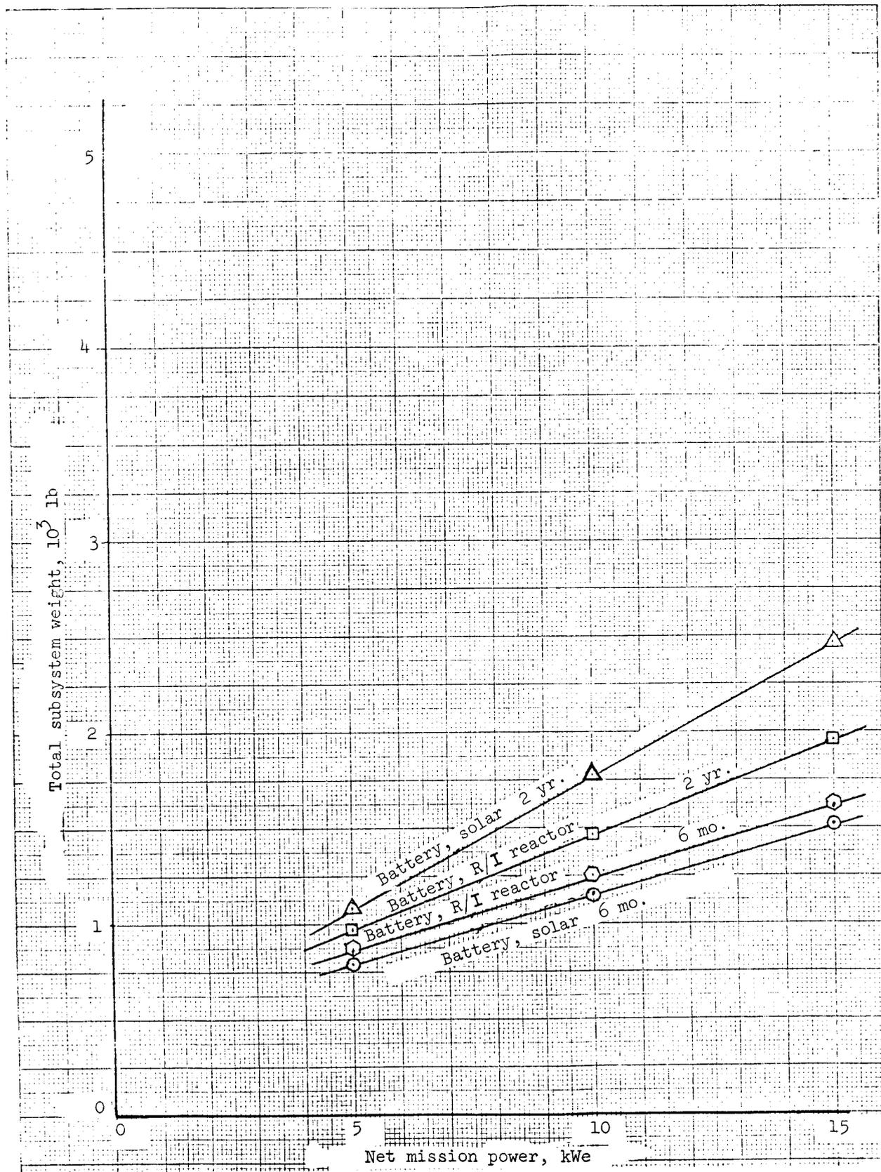
Figure 1.27 . - Synchronous Earth orbit battery supplementary power subsystems.
