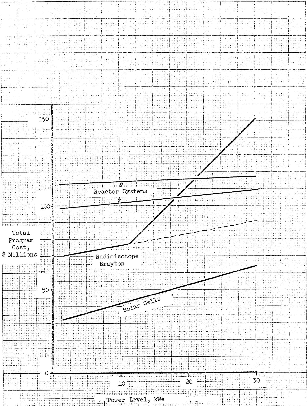
Figure 1.105. - Power system program cost versus power level
