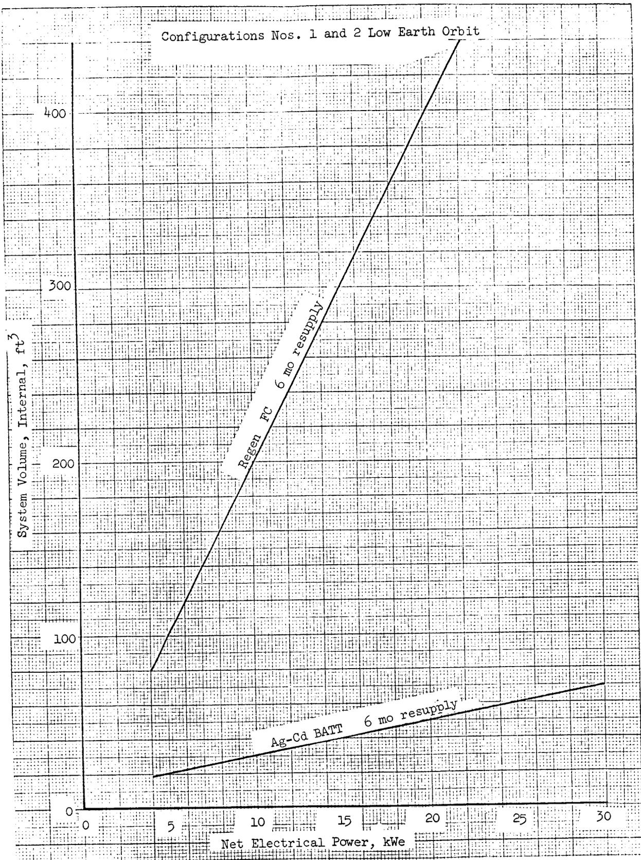
Figure 1.101 - Secondary power system volume versus net electrical power, LEO
