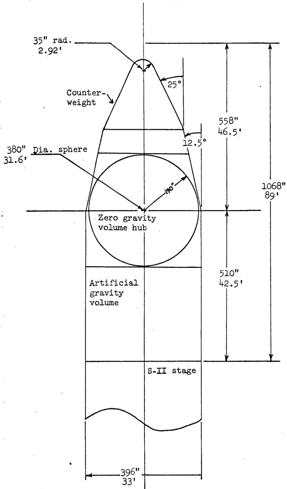
Figure 1-2 - Configuration no. 1, dumbbell space station, launch.
