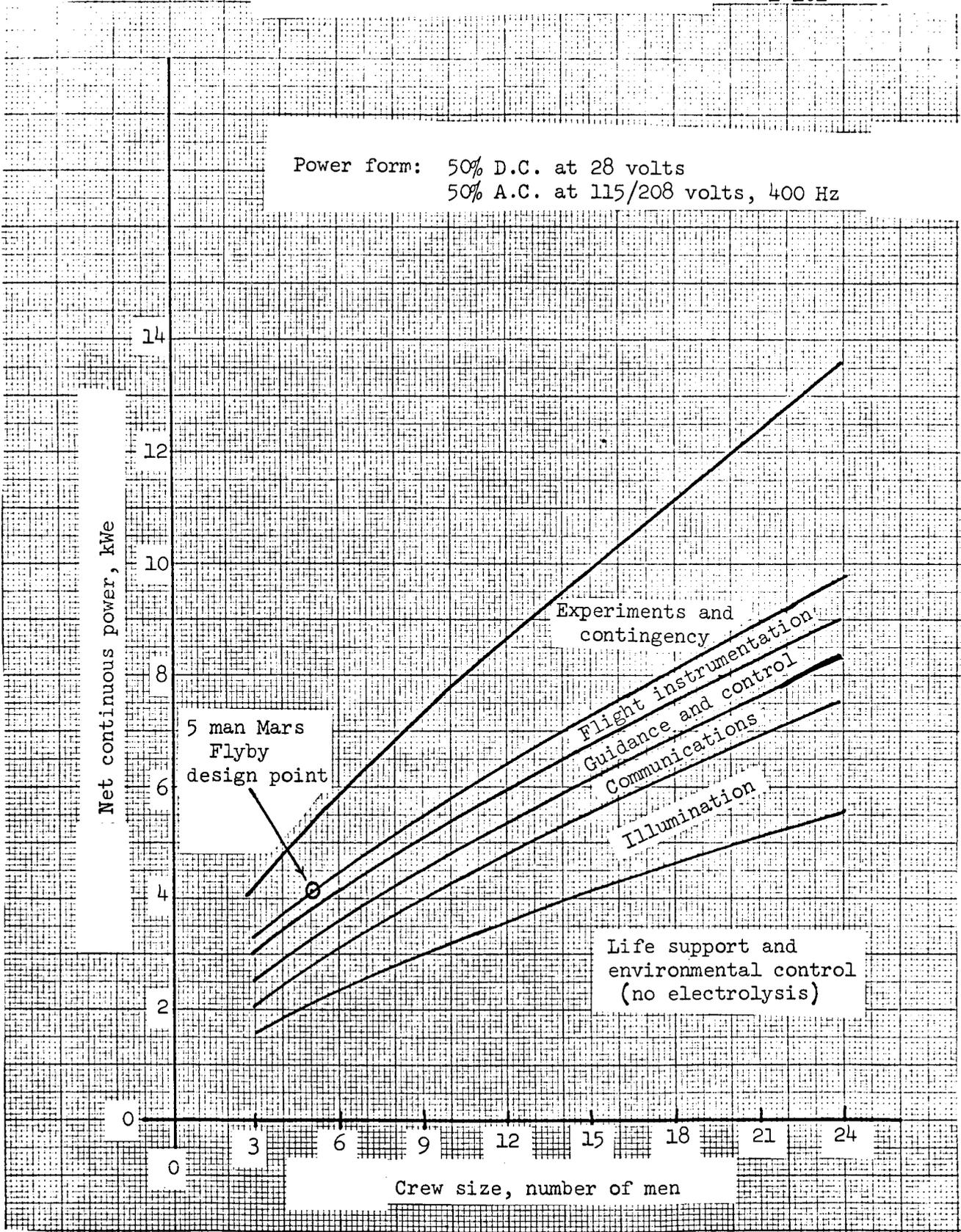
Figure 1.7 - Space station continuous power requirements versus crew size.
