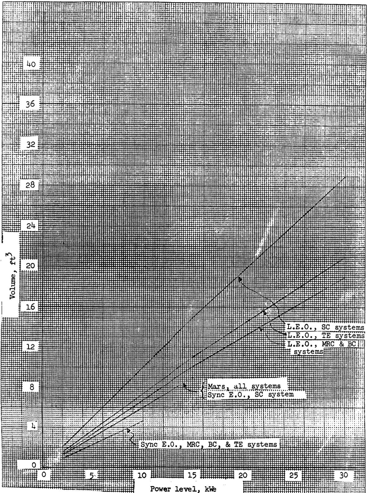
Figure 1.40 - Power conditioning volumes versus power level.
