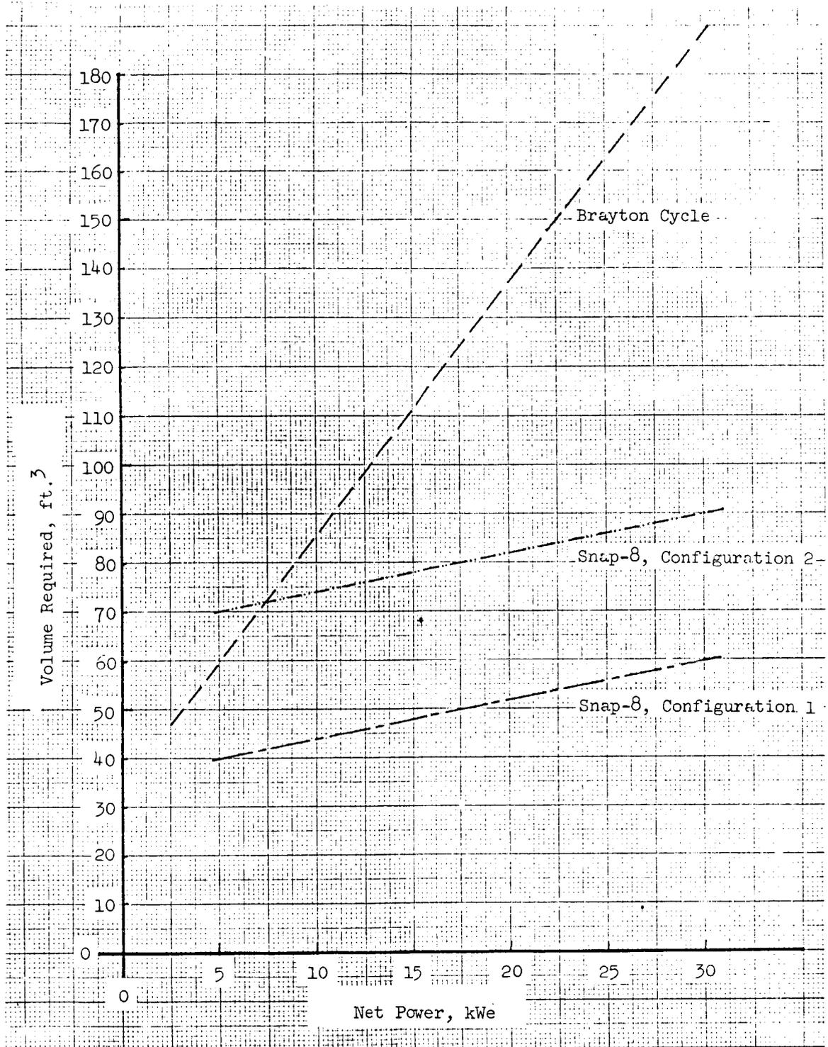
Figure 1-72 - Volume required versus net power for Brayton-cycle systems.
