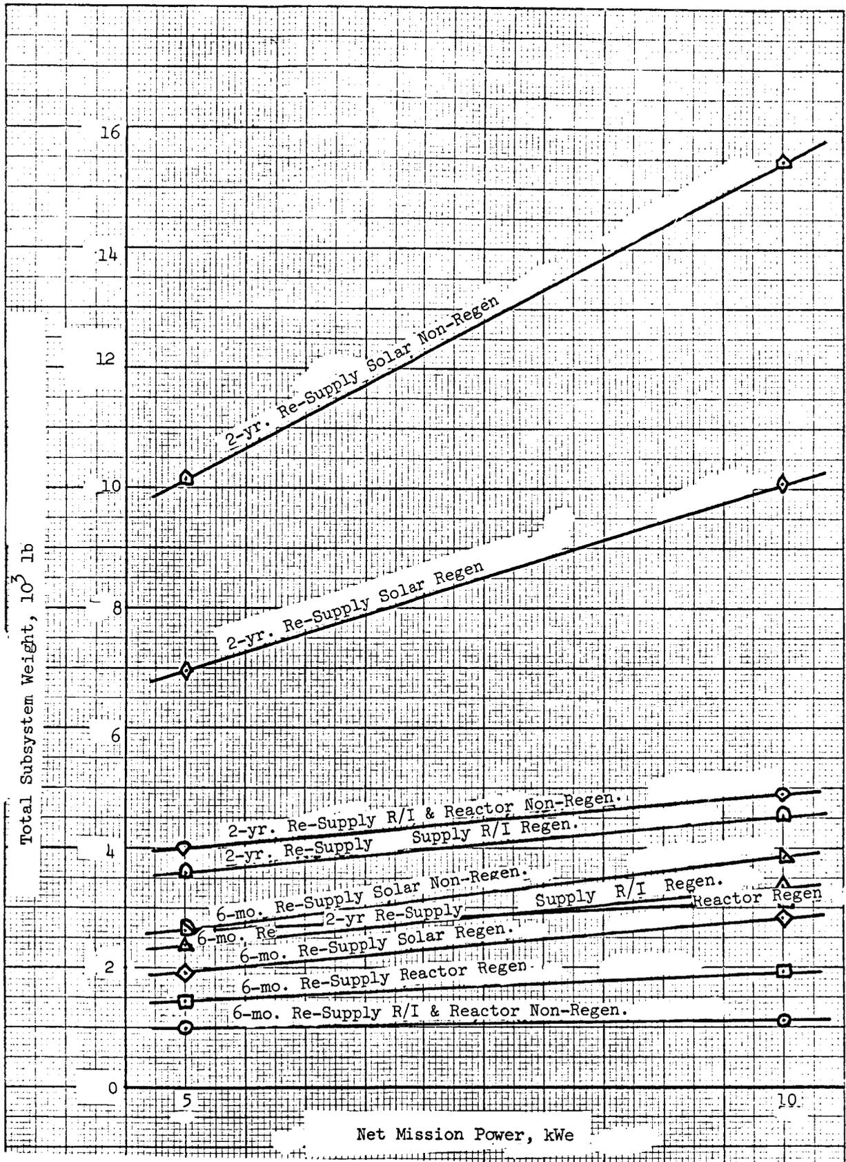
Figure 1.34 - Synchronous Earth orbit fuel cell supplementary power subsystem.
