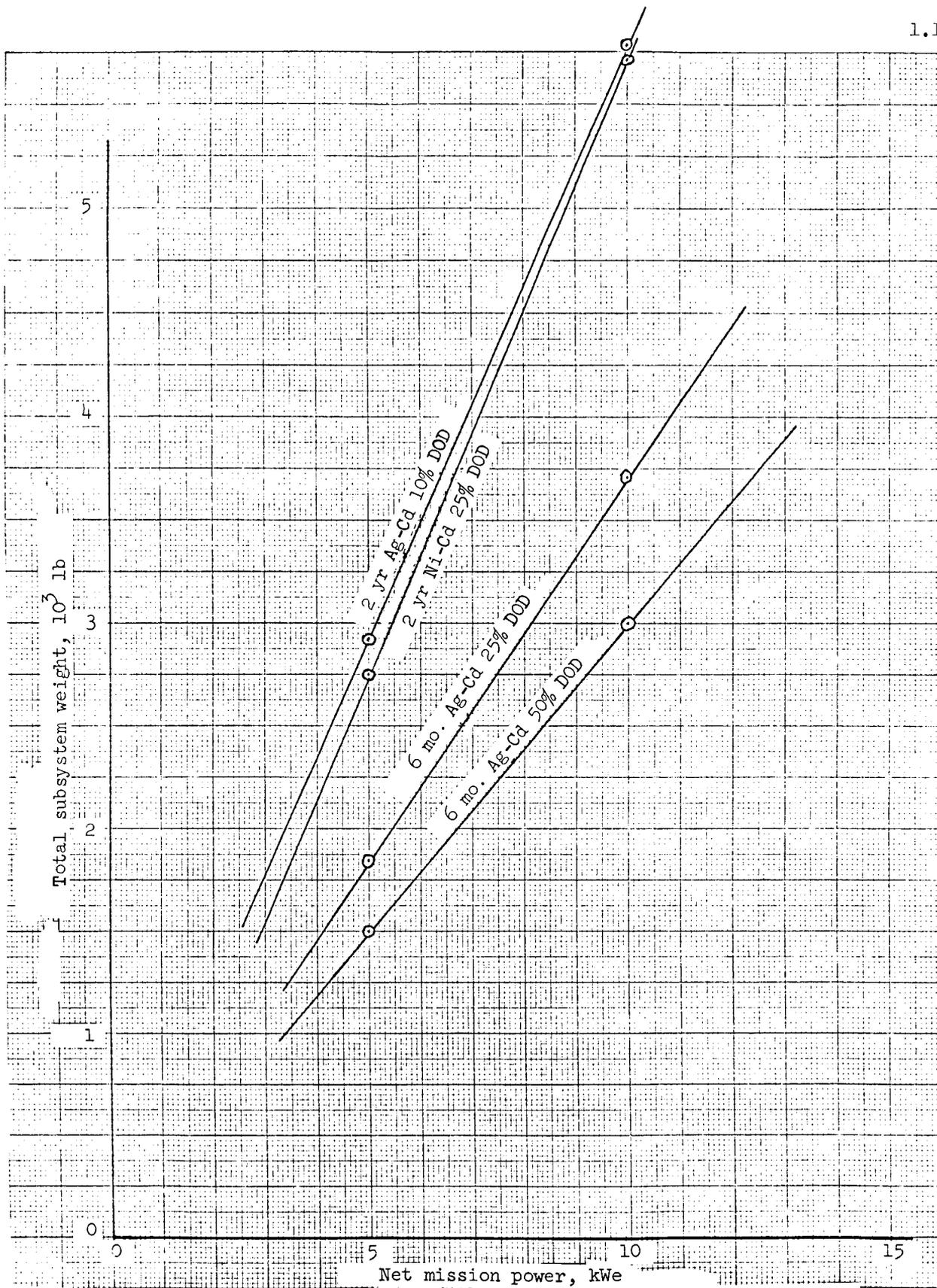
Figure 1.25 - Low Earth orbit battery complementary power subsystems.
