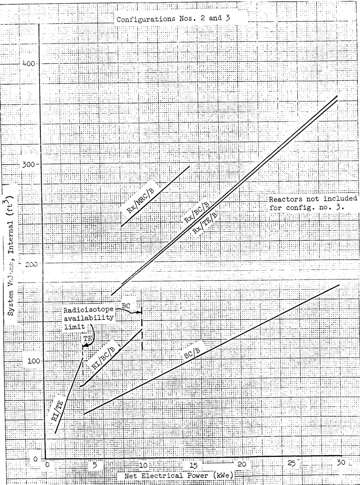
Figure 1.99 - Power system volume versus net electrical power, LEO no. 2 and sync
