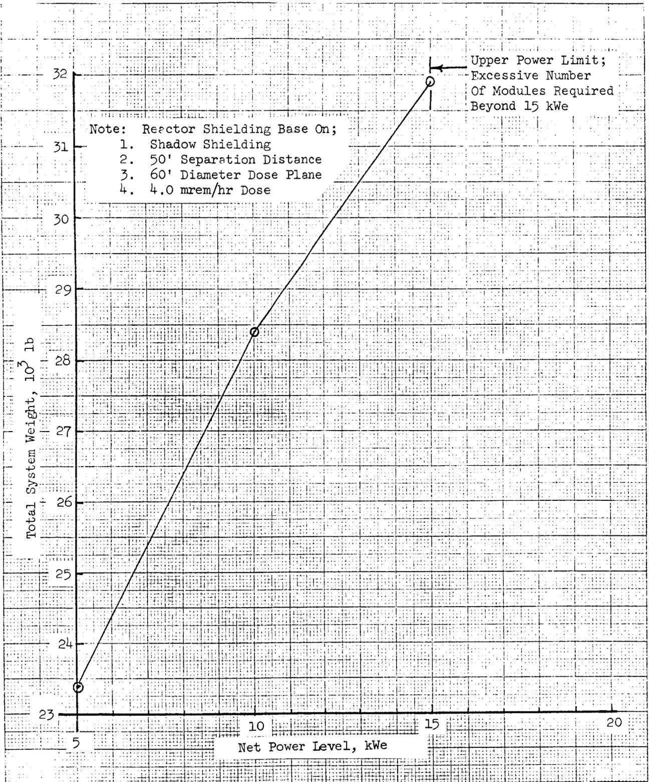
Figure 1.76 - Zero-G Space Station: Total system weight versus net power level for reactor mercury-Rankine systems.
