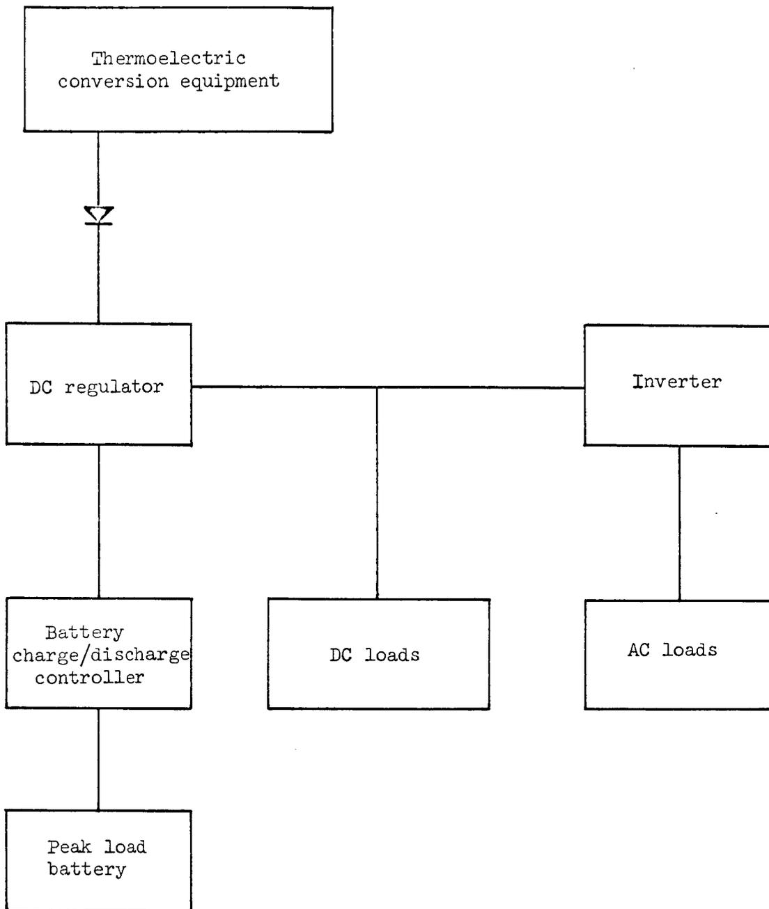
Figure 1.67. - Thermoelectric electrical schematic.
