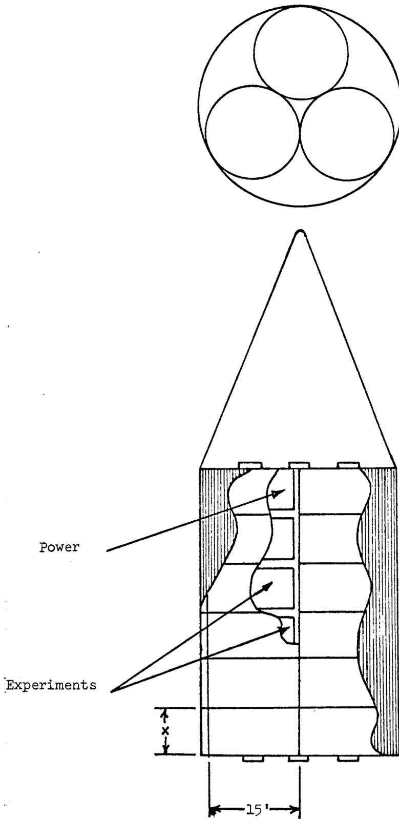
Figure 1-3 - Configuration no. 2, zero-g space station.
