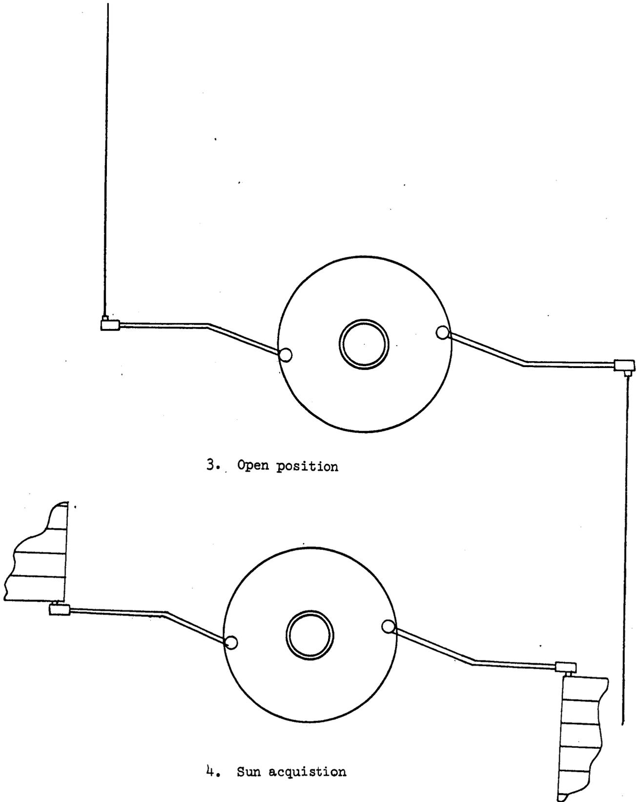
Figure 1.56 - Solar array deployment sequences 3 and 4.
