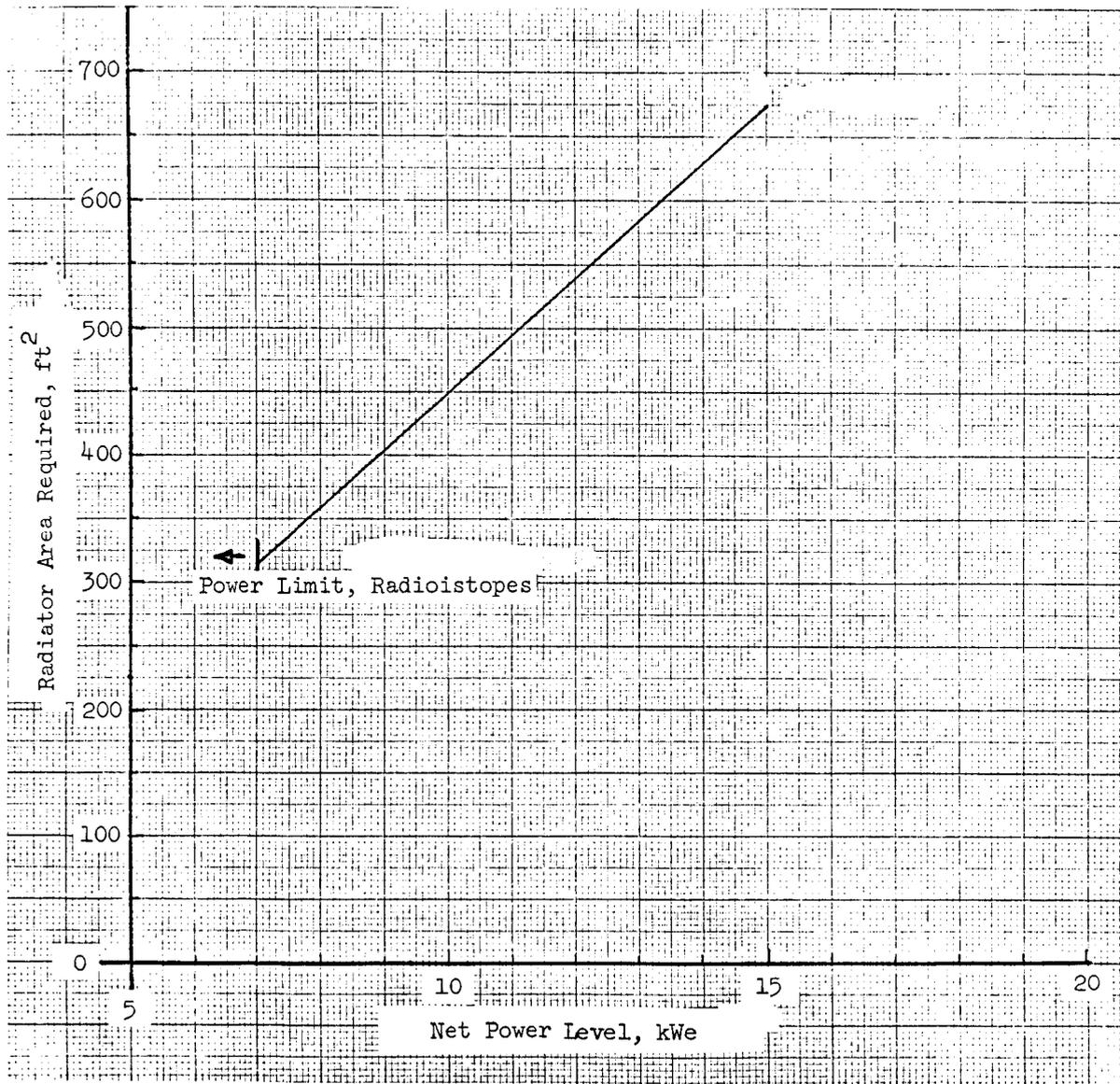
Figure 1-75 - Radiator area required versus net power level for radioisotope and reactor systems using mercury-Rankine.
