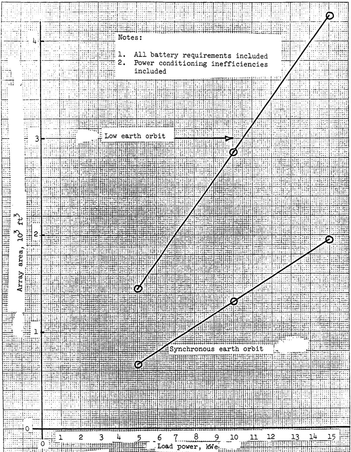
Figure 1.44 - Array area versus power for Earth orbit.
