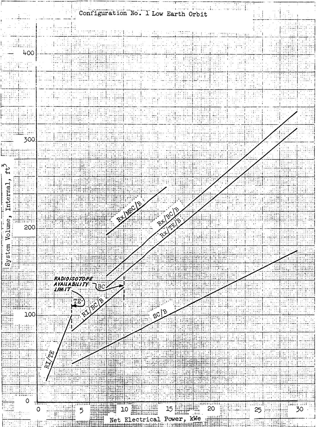
Figure 1.98 Power system volume versus net electrical power, LEO no. 1
