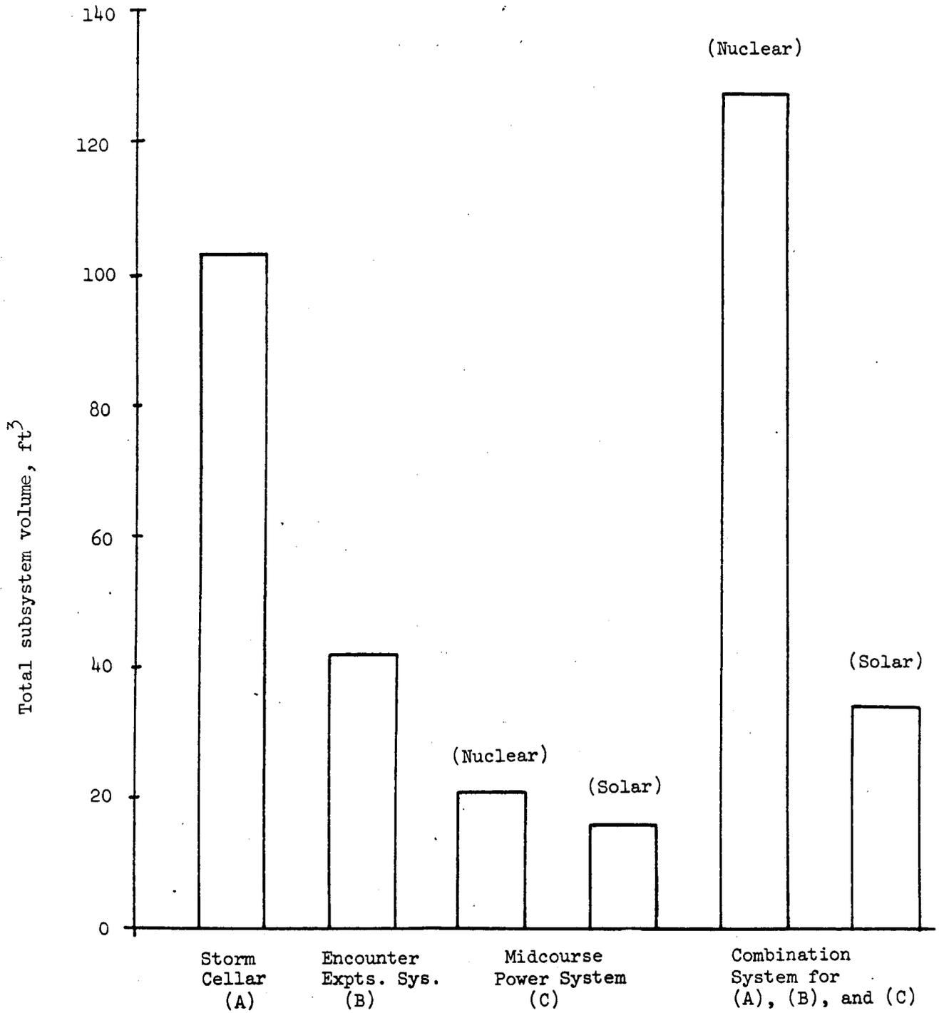
Figure 1.36 - Mars flyby fuel cell power subsystems volume.
