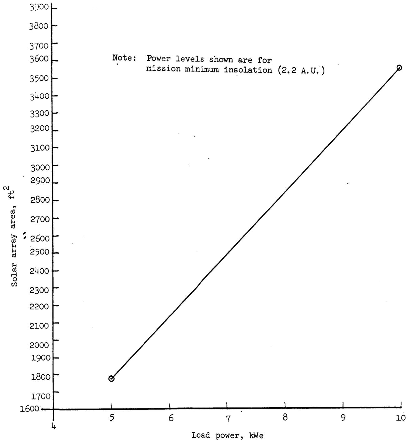
Figure 1.48 - Array area required for a Mars flyby.
