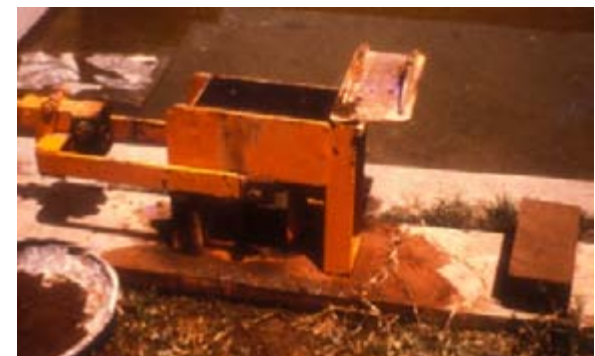
fig. 33 Using a hand-operated press can considerably increase the strength of the brick [Mackenzie 1987]
