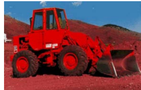
fig.128 front end loader 1 m 3 bucket -> 6000kg machine mass cycle time 30 sec -> 2 m 3 /min
