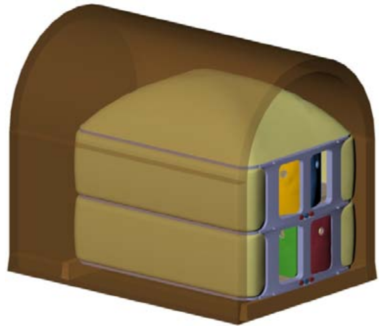
fig. 105 Rear view of one inflatable module inside its masonry protection
