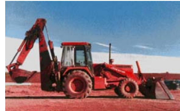
fig. 127 hydraulic excavator (backhoe) 0.4 m 3 bucket -> 10,000 kg machine mass cycle time 15 sec -> 1.6 m 3 /min
