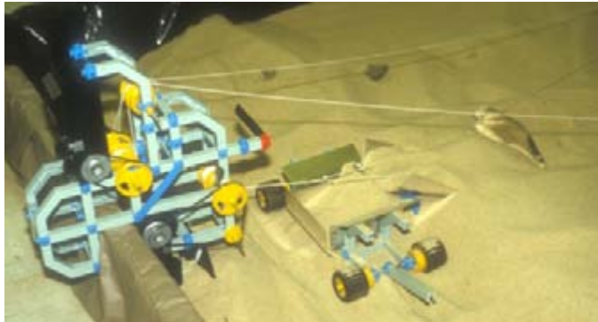
fig. 125 Slusher mock-up built by a team lead by Greg Maryniak at MIT during a lab at the International Space University in 1988.
