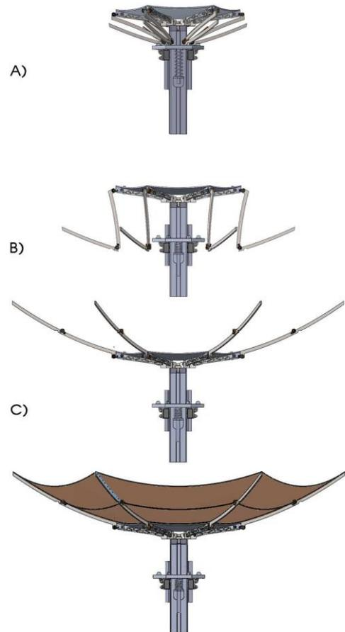
Figure 2: Deployment sequence, A, B, C not representative of the membrane.
