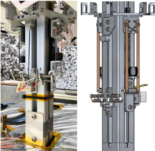
Figure 4: CDR design and final configuration of the actuation subsystem.
