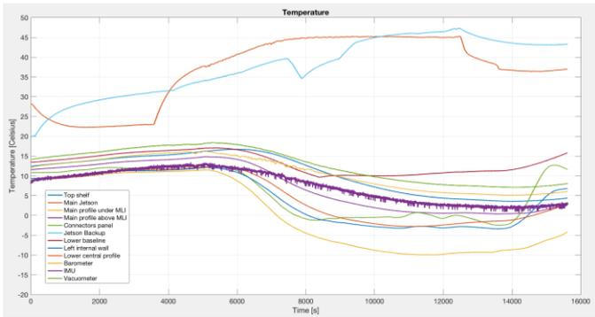
Figure 6: Temperature profiles of several components during BEXUS-24 flight.
